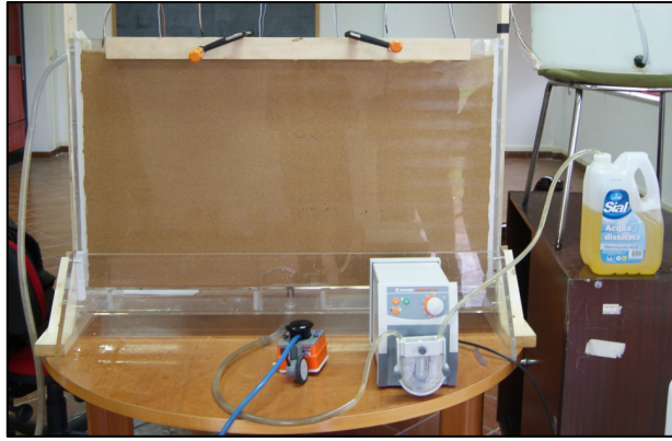
Figure 2. 11: Hydrocarbon injection by means of a peristaltic pump
