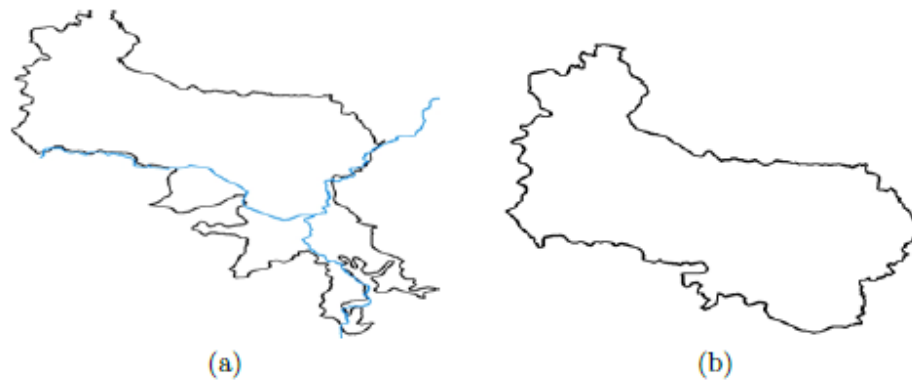
Figure 3. 29: a) Aquifer geological boundaries b) Aquifer modeling boundaries
