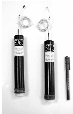
Figure 2. 28: Nonpolarizing Pb/PbCl 2 (Petiau) electrodes
