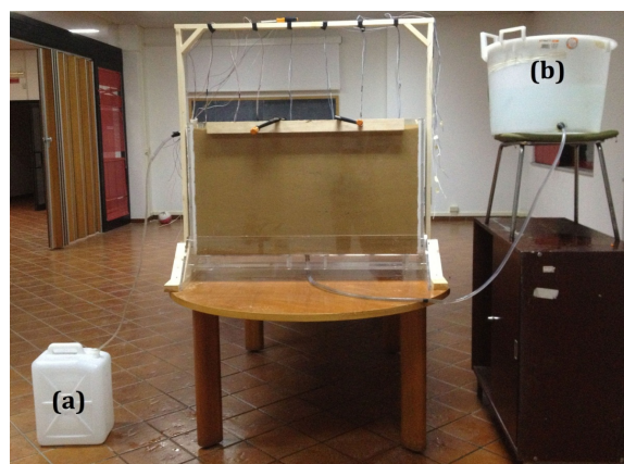
Figure 2. 10: Hydraulic loading system: (a) collection tank; (b) loading tank.
