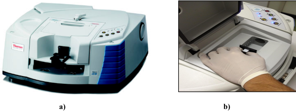
Figure 2. 16: a) Infrared Spectrophotometry Thermo FT-IR Nicolet iS10 b) LNPL samples analysis
