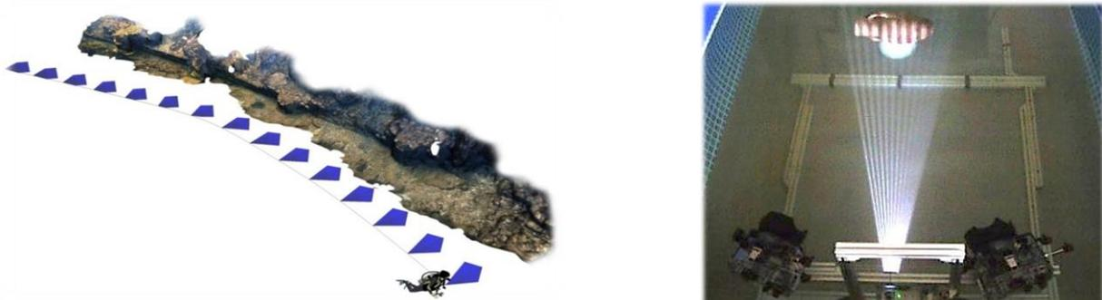
*Figure II-6 Examples of acquisition by passive technique (left) and active technique (right).*
