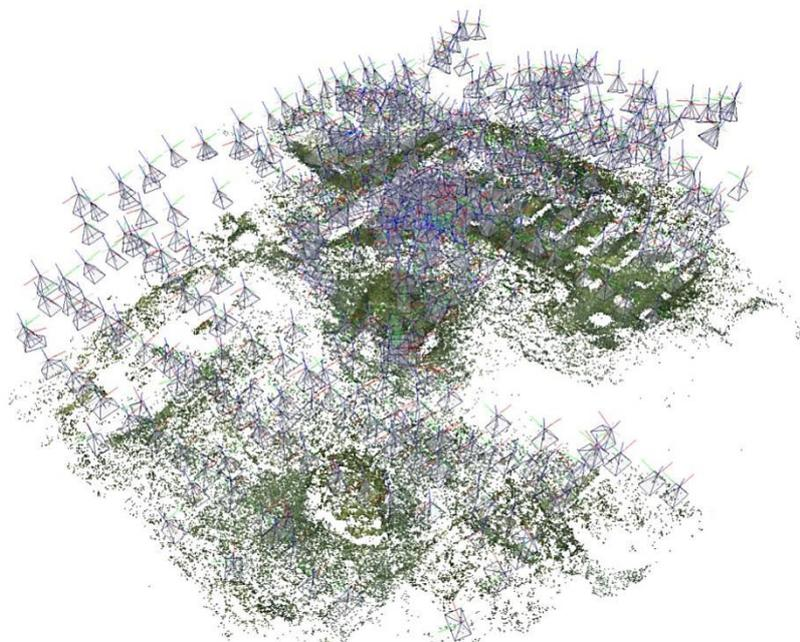
*Figure III-7 Sparse point cloud and 533 oriented frames.*
