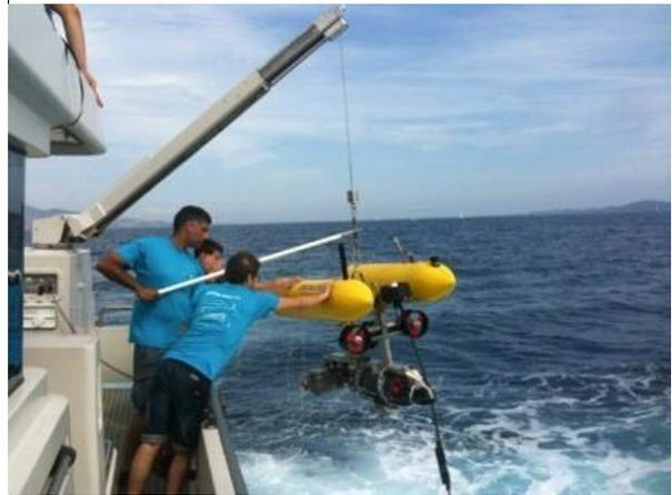
Figure V-10 Left: Schema of the Girona 500 AUV, showing the location of principal components and payload area. Right: Deploying of the Girona 500 AUV above the La Lune shipwreck.
