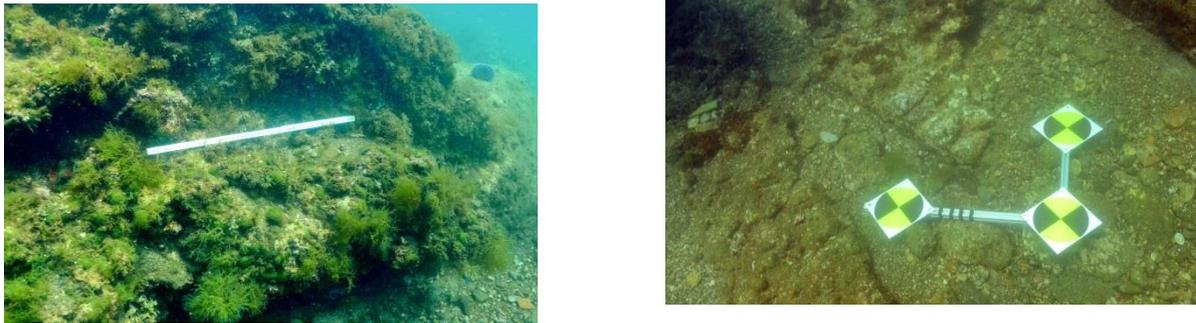
*Figure III-18 The scale bar and a marker over the two areas selected to test the documentation process.*
