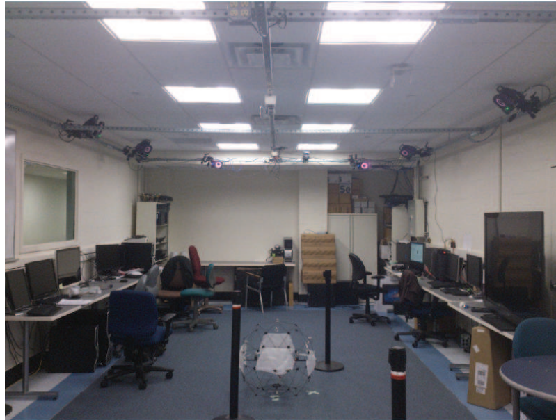
Fig. 5.6. Robust System Lab at Northeastern University: Vicon camera system and Qball-X4
