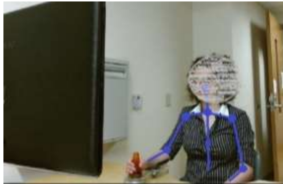
Figure 4.3 A Kinect sensor was placed on the left side of the monitor. A frame taken by the sensor in this configuration is showed. A subject holding the end-effector of the haptic interface, in front of the monitor, and the skeleton tracked by the Kinect are represented.
