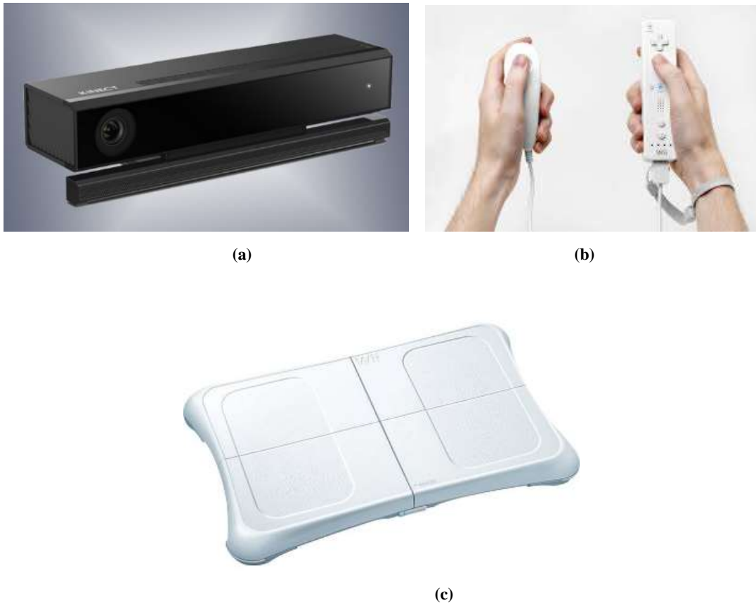
Figure 1.5 Motion controllers. (a) Kinect for Windows by Microsoft; (b) Nintendo Wii; (c) Nintendo wiiFit Balance Board.
