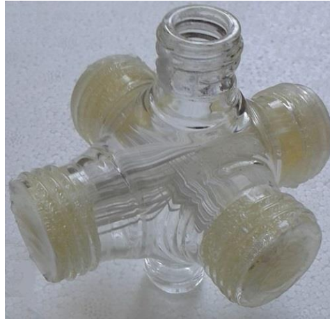
Fig. 2.2. The crossed hollow-fiber membrane bioreactor glass housing with PES hollow-fiber membranes cross assembled into a tight mesh.
