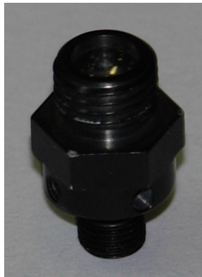
Figure 2-4: The lens that collects the luminescence signal
