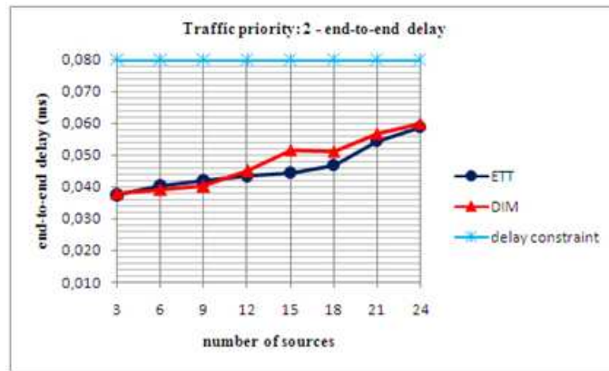
Fig. 4.14. End-to-end delay for traffic classes with priority value equal to "2"
