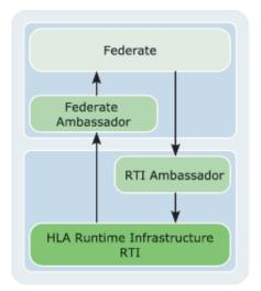
Fig. 2.5. Interfaces between RTI and federates
