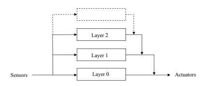
Fig. 1.3. Subsumption architecture layers
