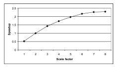
Fig. 3.18. Simulation speedup vs. scale factor (three processors)
