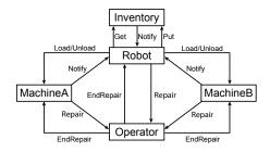
Fig. 4.1. A manufacturing system model
