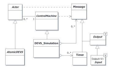
Fig. 4.11. UML Class Diagram of ActorDEVS basic Framework
