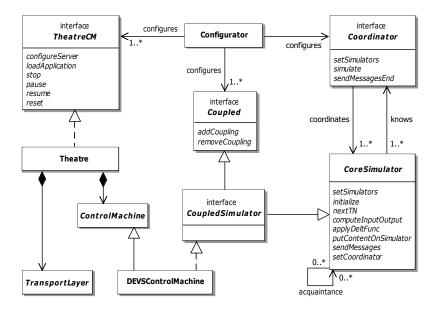
Fig. 4.15. Class diagram of system components
