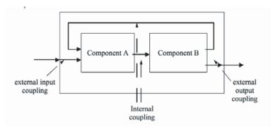
Fig. 2.1. Schema of a coupled model
