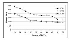
Fig. 3.14. Mission time vs. deployed UAVs
