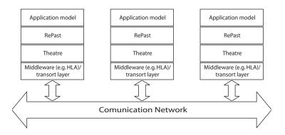
Fig. 6.12. Architecture of a distributed RePast model
