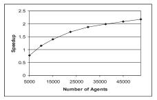
Fig. 6.21. Simulation speedup vs. number of agents (three processors)  $\,$
