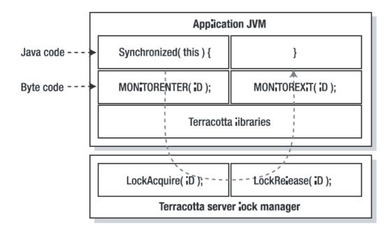
Fig. 2.8. Terracotta hooks into the MONITORENTER and MONITOREXIT bytecodes
