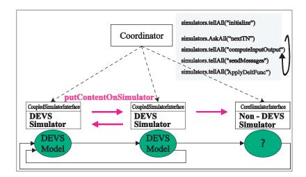
Fig. 4.13. Simulation protocol in a federation of DEVS and non-DEVS simulators
