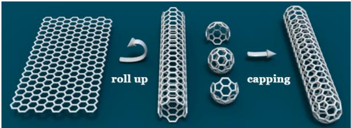
Fig. 3.2. Carbon SWNT structure
