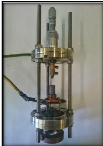
Figure 5.4: Apparatus assembled to synthesis of CNOs by arc discharge in water.
