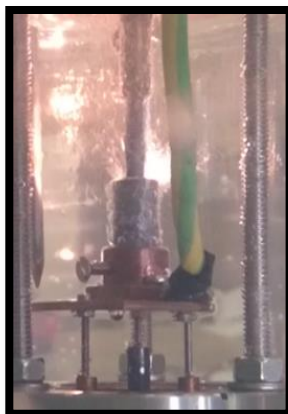
Figure 5.6: Digital image of the experimental process during arc discharge between anode and cathode of graphite.
