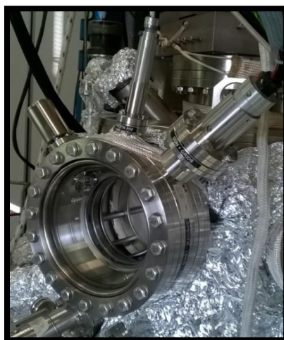
Figure 2.2: Picture of low energy electron diffraction apparatus.
