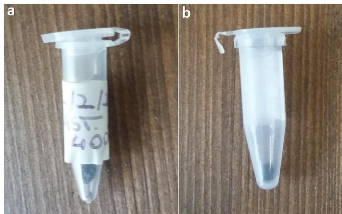
Figure 5.10: Agglomerates formed on the cathode, a) heated to 400 °C, b) without heating.
