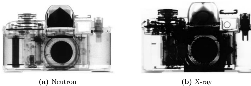
Figure 2.3: Comparison between radiographs [12] obtained with neutrons (a) and X-rays (b).
