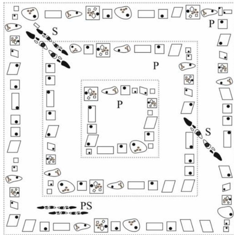
Figure 3.2. Idealized distribution of primary (P), secondary (S) and pseudo-secondary (PS) fluid inclusions showing different type and shape in halite crystal (right).
