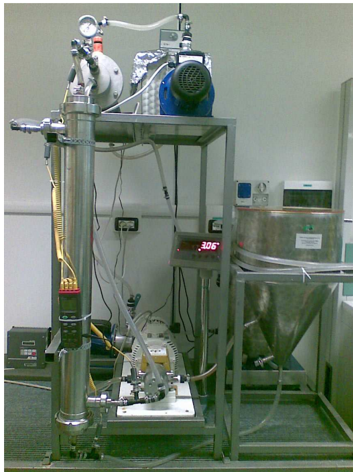
Figure 6.3 The MD/MDC plant
