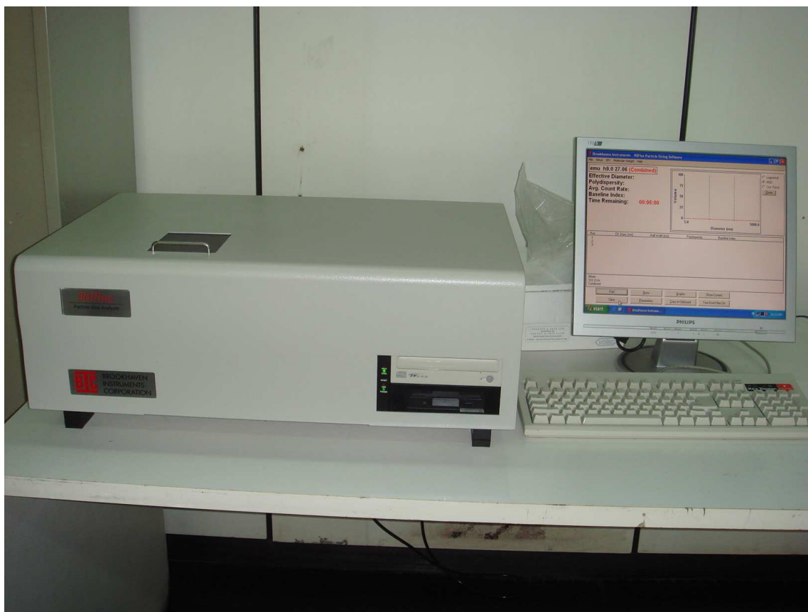
Figure 2.12 The DLS device
