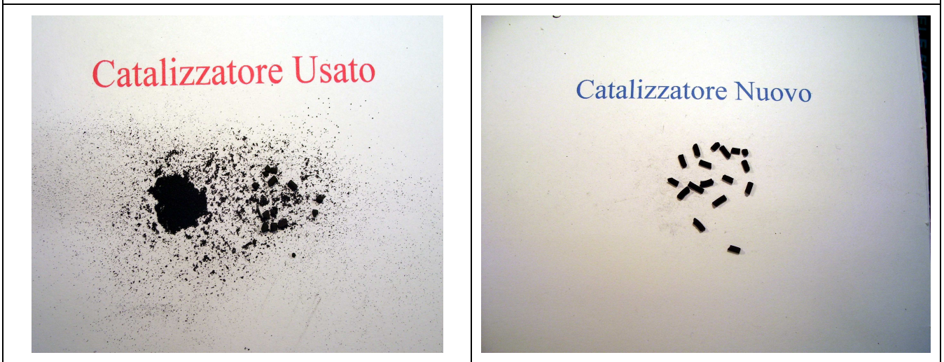
Fig. 59 – Catalyst exhausted after an experimental tests cycle and fresh catalyst, respectively.
