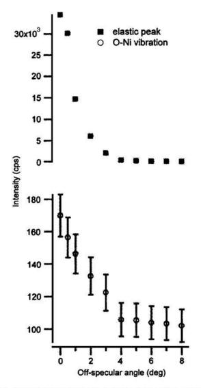
FIG. 4. Behavior of the intensity of the elastic beam and of the vibrational loss of oxygen as a function of the off-specular angle suggesting the dipolar character of the O–Ni peak.
