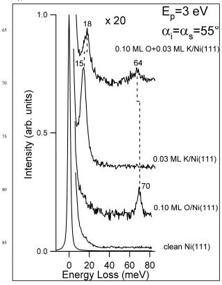
90 Figure 2. HREEL spectra of: (a) 0.03 ML of K deposited at 400 K onto the Ni(111) surface; (b) 0.10 ML O/Ni(111) at the same temperature; (c) 0.03 ML K coadsorbed at 400 K with 0.10 ML of O on the Ni(111) surface.
