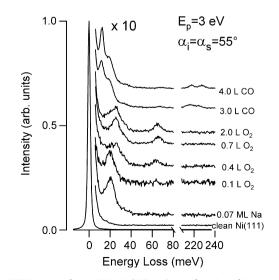
Fig. 7. HREEL spectra for 0.07 ML Na/Ni(111) as a function of  $O_2$  exposure (at 400 K) and of successive CO exposure (at room temperature).
