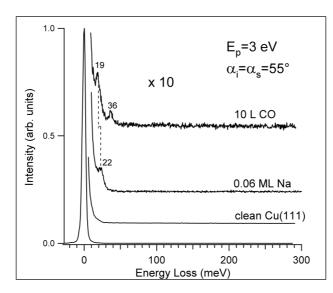
Figure 2: HREEL spectra for 0.06 ML Na/Cu(111) exposed to CO molecules at room temperature.
