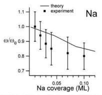
**Figure 5.** Comparison between the theoretical behavior of the A–S stretching vibration (data taken from ref 27, with permission) and the experimental curve for Na reported in Figure 3a. The frequency of the A–S stretching,  $\omega$ , was normalized to its value for the lowest alkali coverage,  $\omega_0$ .
