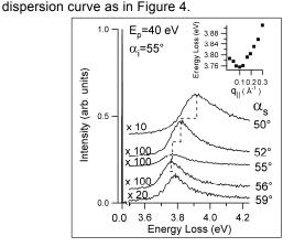
Figure 5: HREEL spectra for 22 ML Ag/Cu(111) as a function of the scattering angle after an annealing at 400 K. In the inset the dispersion relation of the Ag SP energy is shown. The initial flat behavior reported in Figure 4 abruptly changed upon annealing and an initial negative dispersion appeared .
