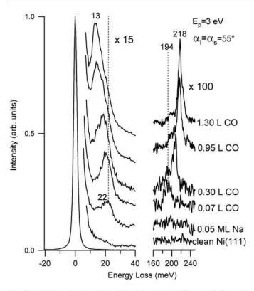
Fig. 2 HREEL spectra for 0.05 ML Na/Ni(111) at 400 K for different CO exposures at room temperature
