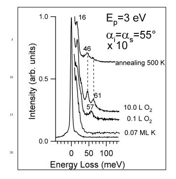
*Figure 1.* HREEL spectra of 0.07 ML of K deposited on Cu(111) at 400 K and successively exposed to O<sub>2</sub>. Both O<sub>2</sub> exposures and measurements were carried out at 400 K. All spectra were multiplied by the same factor.
