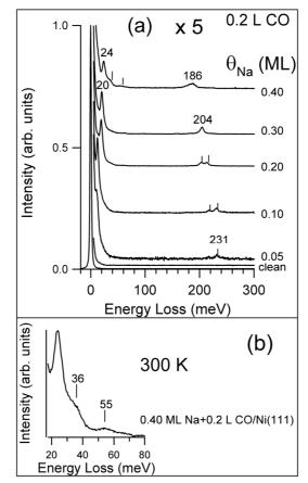
Figure 4: (a) HREEL spectra of various coverages of Na deposited onto the Ni(111) surface at 300 K and exposed to 0.2 L of CO at the same temperature; (b) Magnification of the spectrum of 0.40 ML Na/Ni(111). Two loss features at 36 meV (O-Na) and 55 meV (C-Na) were recorded.
