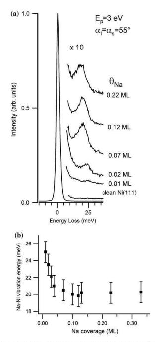
**Fig. 1** (a) HREEL spectra of Na deposited at 400 K onto the Ni(111) surface as a function of the alkali coverage. (b) Na–Ni vibration energy as a function of the Na coverage
