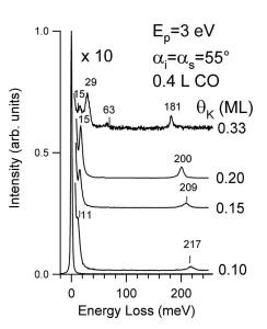
FIG. 4. HREEL spectra of various coverages of K deposited onto the Ni(111) surface at 300 K and exposed to 0.4 L of CO at the same temperature. The appearance of loss features at 29 and 63 meV, ascribed to the O–K and the O–Ni vibrations, respectively, indicates the partial dissociation of CO molecules.
