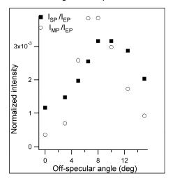
Figure 11: Behavior of the ratio of the intensity of the SP with respect to that of the elastic peak,  $I_{SP}/I_{EL}$ , and of the ratio of the intensity of the MP with respect to that of the EP peak,  $I_{MP}/I_{EP}$ , as a function of the off-specular angle. A maximum for both quantities was found around seven-eight degrees off-specular. For such angle, the intensity of MP was higher than that of the SP peak.
