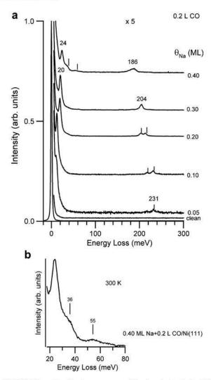
Fig. 3. (a) HREEL spectra of various coverages of Na deposited onto the Ni(111) surface at 300 K and exposed to 0.2 L of CO at the same temperature; (b) Magnification of the spectrum of 0.40 ML Na/Ni(111). Two loss features at 36 meV (O–Na) and 55 meV (C–Na) were recorded.
