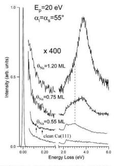
Fig. 2. HREELS spectra of the Cu(111) surface and for  $\theta_{Na} = 0.55$ , 0.75 and 1.20 ML.
