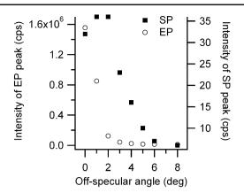
**Fig. 4** Intensity of the SP and of the elastic peak (*EP*) as a function of the off-specular angle
