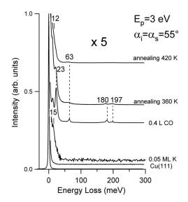
FIG. 1. HREEL spectra for 0.05 ML K deposited at 400 K on Cu(111) and exposed to CO at 300 K. Measurements were carried out at 300 K. All spectra were multiplied by the same factor. The intensity of all peaks was normalized to that of the elastic peak.
