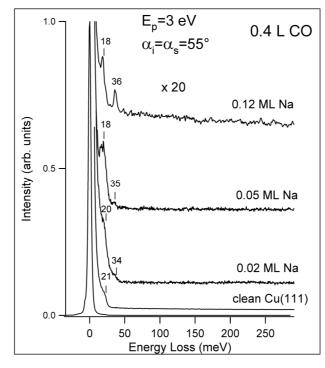
Figure 3: HREEL spectra for different amounts of Na deposited onto the Cu(111) surface and successively exposed to 0.4 L of CO. No critical precoverage for CO dissociation exists. The peak at 21 meV recorded for the clean Cu(111) surface is assigned to the copper optical phonon [50].
