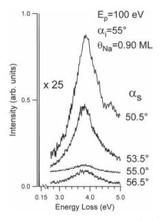
Fig. 3. Electron energy loss spectra of 0.90 ML Na/Cu(111) at different scattering angles  $\theta_s$ , recorded with a primary electron beam energy of 100 eV.
