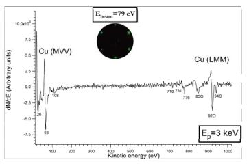
Figure 2: AES spectrum of the clean Cu(111) surface. The correspondent LEED pattern is also shown.
