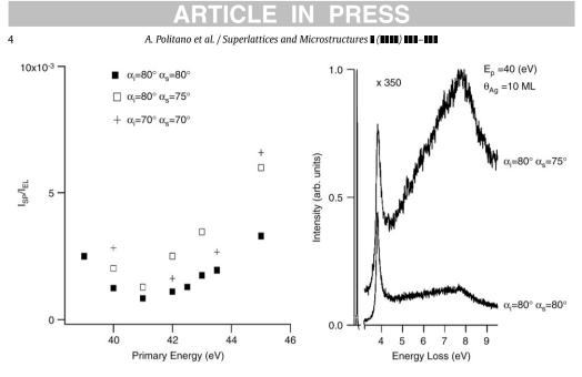
Fig. 3. (Left): Behavior of the intensity of the SP peak as a function of the impinging energy for different scattering geometries in grazing conditions. All intensities were normalized to that of the elastic peak. (Right) Besides the ordinary surface plasmon, a loss feature at 7.5 eV was excited in spectra recorded at grazing incidence. Its enhanced intensity in off-specular spectra ensures its impact character.
