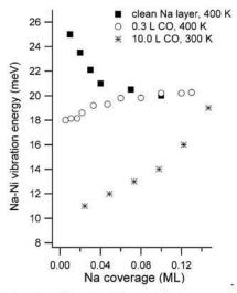
Figure 4. Behavior of the Na-Ni stretching energy for a clean Na adlayer and for Na dosed onto a CO-modified Ni(111) surface at 400 and 300 K, respectively.
