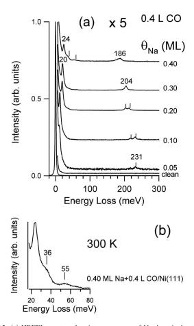
FIG. 5. (a) HREEL spectra of various coverages of Na deposited onto the Ni(111) surface at 300 K and exposed to 0.4 L of CO at the same temperature. (b) Magnification of the spectrum of 0.40 ML Na/Ni(111). Two loss features at 36 meV (O–Na) and 55 meV (C–Na) were recorded.
