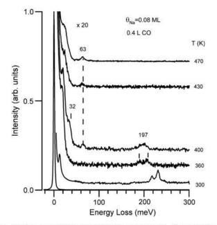
**Fig. 1.** HREEL spectra of 0.08 ML Na/Ni(111) exposed to 0.4 L CO as a function of the sample temperature. Na deposition and CO exposure were made at the same temperature. CO adsorption was found to be partly dissociative at 400 K and co-mpletely dissociative for temperatures higher than 430 K. The intensity of all peaks was normalized to the intensity of the elastic peak. All spectra were multiplied by the same factor.
