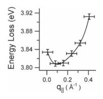
**Fig. 5.** Na SP energy as a function of  $q_{\parallel}$  ( $E_{p} = 100 \text{ eV}$ ).
