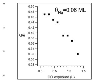
Figure 7: The dynamic dipole charge Q/e (e is the electron charge) of Na as a function of CO exposure.
