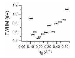
**Fig. 7.** FWHM of the Na SP peak as a function of  $q_{\parallel}$  ( $E_p = 20$  eV).
