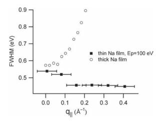
**Fig. 8.** FWHM of the Na SP peak as a function of  $q_{\parallel}$  for ( $\blacksquare$ ) 0.90 ML Na/Cu(111),  $E_p = 100$  eV and for (o) thick Na film (data taken from Ref. 10).
