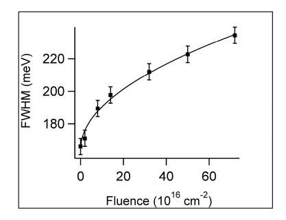
Figure 2: Behavior of the FWHM as a function of the fluence of the  $Ar^+$  ion beam.
