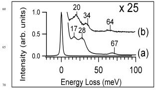
Figure 8. HREEL spectrum acquired for 0.10 ML K deposited onto a 0.10 ML O-modified Ni(111) surface (spectrum a). Reversing the order of adsorption, the alkali-O bond is formed. Similar results were obtained by substituting K with Na (spectrum b).
