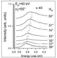
Figure 3: HREEL spectra for 22 ML Ag/Cu(111).
