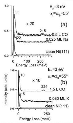
Figure 2. HREEL spectra of Na (panel a) and K (panel b) deposited on Ni(111) at 400 K and after the exposure of the alkali layer to CO at room temperature.
