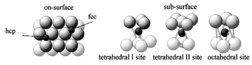
Figure 5: On-surface and subsurface adsorption sites [58]
