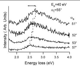
**Fig. 2** HREEL spectra of the Au(111) film as a function of the scattering angle. A clear dispersion of energy of the broad loss peak, assigned to the Au SP, exists, as indicated by the *arrow*
