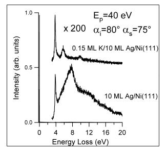
Figure 12: HREEL spectra of 10 ML Ag/Ni(111) after the exposure of 0.15 ML of K at room temperature. MP disappeared and new loss features due to water contamination arose in spectrum.
