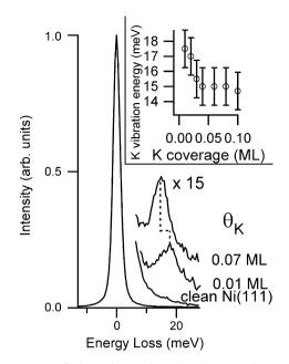
**Fig. 2.** HREEL spectra of K layers deposited on Ni(1 1 1) at 400 K (loss spectra were acquired at the same temperature). The inset shows the behaviour of the K-substrate vibration as a function of K coverage.
