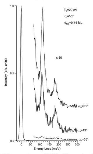
Fig. 3. Electron energy loss spectra of Cu(111) at different scattering angles  $\alpha_s$ . The incident beam energy  $E_p$  is held constant at 20 eV and all spectra were recorded at an incident angle of  $\alpha_i = 55^\circ$  with respect to the sample normal.
