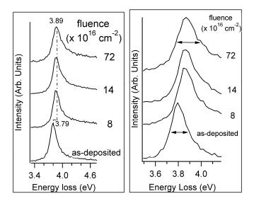
Figure 1: (left panel) HREEL spectra for 10 layers of Ag/Cu(111). The SP energy shifted from 3.79 eV (as-deposited film) to 3.89 eV, regardless of fluence. On the other hand, the FWHM of the SP peak broadened upon sputtering; (right panel) HREEL spectra after the subtraction of a polynomial background, presented in a restricted energy range. The arrows indicate the value of the FWHM, which increased from 164 to 235 meV upon increasing the fluence.
