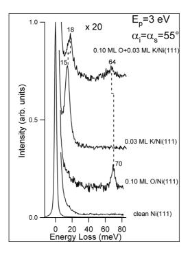
Figure 10: HREEL spectra of: (a) 0.03 ML of K deposited at 400 K onto the Ni(111) surface (b) 0.10 ML O/Ni(111) at the same temperature (c) 0.03 ML K coadsorbed at 400 K with 0.10 ML of O on the Ni(111) surface.
