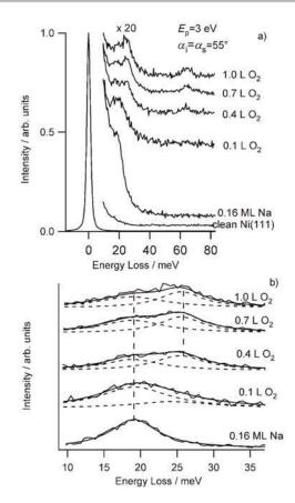
Figure 4. a) HREEL spectra of Ni(111) and 0.16 ML Na/Ni(111) exposed to  $O_2$  molecules at 400 K. b) Each curve is obtained using the same procedure as Figure 1 b.
