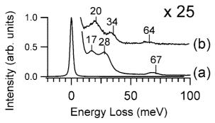
**Figure 3.** HREEL spectrum acquired for 0.10 ML K deposited onto a 0.10 ML O-modified Ni(111) surface (spectrum a). Reversing the order of adsorption, the alkali–O bond is formed. Similar results were obtained by substituting K with Na (spectrum b).
