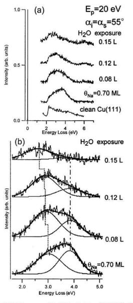
FIG. 2. (a) HREEL spectra of Cu(111) and of  $\theta_{Na}$ =0.55 ML/Cu(111) exposed to water vapor. Na Mie resonance is at 3.0 eV. (b) Each curve was obtained by subtracting the background and the copper contribution. The resulting curve was fitted by a Gaussian line shape.
