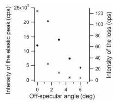
**Fig. 10.** Intensity of the SP (•) and of the elastic peak (\*) as a function of the off-specular angle  $(E_p = 100 \text{ eV})$ .
