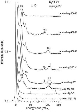
**Fig. 2.** HREEL spectra of 0.50 ML Na/c-( $4 \times 2$ )-CO/Ni(111) at 200 K. Annealing at progressively higher sample temperature caused CO dissociation and the desorption of CO molecules and O-derived species.
