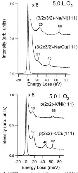
**Figure 2.** HREEL spectra (at a fixed O<sub>2</sub> exposure of 5.0 L) for (top panel)  $(3/2 \times 3/2)$ -Na/Cu(111) and  $(3/2 \times 3/2)$ -Na/Ni(111); (bottom panel) p(2 × 2)-K/Cu(111) and p(2 × 2)-K/Ni(111).
