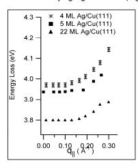
Figure 4: Dispersion of the SP energy for different Ag coverages. The lack of a dispersion before a critical wave-vector indicates that the SP is confined within Ag grains.
