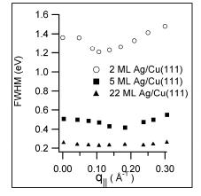
Figure 7: Behavior of the FWHM of the Ag SP as a function of Ag thickness on Cu(111).
