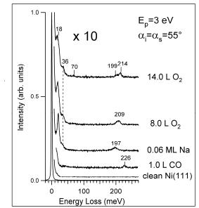
75 Figure 2: HREEL spectra for Na coadsorption with O onto a Ni(111) surface modified by the adsorption of 1.0 L of CO. In this case the Na-O bond was formed, as revealed by the appearance of the feature at 36 meV. In a CO-modified surface, the O-Ni stretching was revealed at 70 meV.
