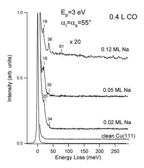
FIG. 3. HREEL spectra for various amounts of Na deposited at 400 K on Cu(111) and exposed to CO at 300 K. The absence of C–O stretching ensures that all CO molecules dissociated. Loss features recorded at 34–36 meV are assigned to the vibration of Na against O adatoms arising from CO dissociation.
