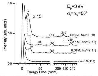
Figure 1. HREEL spectra of (a) 0.06 ML Na deposited at 400 K onto the Ni(111) surface; the loss spectrum was acquired at the same temperature, (b) 0.5 ML CO/Ni(111) dosed at room temperature, (c) 0.06 ML Na coadsorbed with CO at room temperature. All spectra were multiplied by the same factor.
