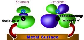
Figure 4: The mechanism for CO adsorption on metal substrates, which implies a back-donation process [35, 36] from  $5\sigma$  to anti-bonding  $2\pi^*$  orbitals of CO, so as to weaken the intramolecular bond of CO molecules.
