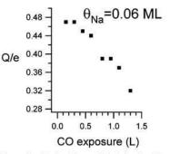
Figure 6. The dynamic dipole charge Q/e (*e* is the electron charge) of Na as a function of CO exposure.
