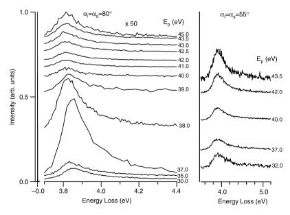
**Fig. 2.** (Left) Magnification of left panel of Fig. 1 around  $E_p = 40$  eV (Right) HREEL spectra for 10 ML Ag/Ni(111) for different primary energies for a scattering geometry far from grazing conditions.
