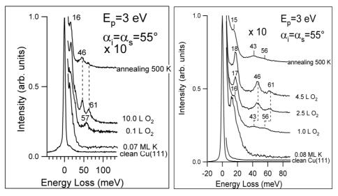
Figure 9: (left panel) HREEL spectra for 0.07 ML K/Cu(111) as a function of  $O_2$  exposure. In the first stage, only subsurface site was populated by oxygen adatoms; (right panel) the same, but for a different K/O ratio. At the saturation the intensity of over-surface O-Cu vibration dominates.
