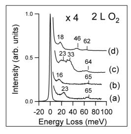
Figure 12: HREEL spectra (at a fixed  $O_2$  exposure of 2 L) for (a) 0.1 ML Na/Cu(111); (b) 0.1 ML K/Ni(111); (c) ( $\sqrt{3}x\sqrt{3}$ )R30°-Na/0.2 ML CO/Ni(111); (d) p(2x2)-K/Cu(111).
