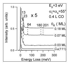
FIG. 6. HREEL spectra for various coverage of K deposited at 400 K on Cu(111) and exposed to CO at 300 K. Measurements were carried out at 300 K. A partial CO dissociation was argued by the presence of O-related modes.
