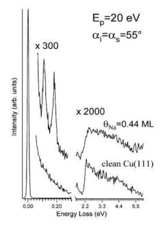
Fig. 1. HREEL spectra of the Cu(111) clean surface and for  $\theta_{\rm Na}\,{=}\,0.44$  ML.
