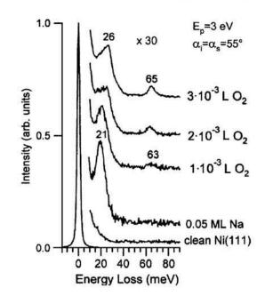
FIG. 1. HREEL spectra for 0.05 ML Na/Ni(111) as a function of  $O_2$  exposures. Upon O adsorption, the Na–Ni vibration energy shifted from 21 to 26 meV.
