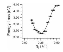
**Fig. 4.** Na SP energy as a function of  $q_{\parallel}$  ( $E_p = 20$  eV).
