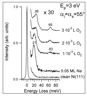
*Figure 4.* HREEL spectra for Na-doped Ni(111) surface: as for K+O/Ni(111) no subsurface oxygen was revealed.
