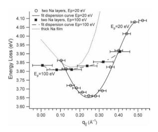
**Fig. 6.** The surface plasmon dispersion versus the parallel momentum  $q_{\parallel}$  for: (**■**) two Na layers,  $E_p = 100 \text{ eV}$ ; (o) two Na layers,  $E_p = 20 \text{ eV}$ ; (-) thick Na film (data taken from Ref. [10]).
