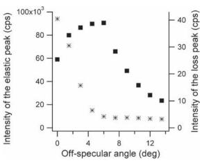
**Fig. 9.** Intensity of the SP ( $\blacksquare$ ) and of the elastic peak (\*) as a function of the off-specular angle ( $E_n = 20$  eV).
