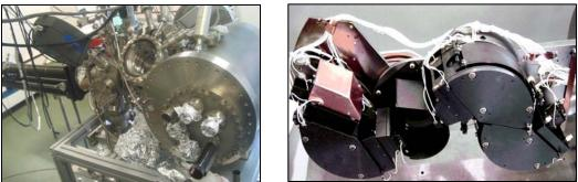
Figure 1: (left panel) UHV chamber used for experiments (right panel) HREELS spectrometer in the straight-trough position. It has a double-step monochromator and a single-step analyzer. Its ultimate energy resolution is 0.5 meV.
