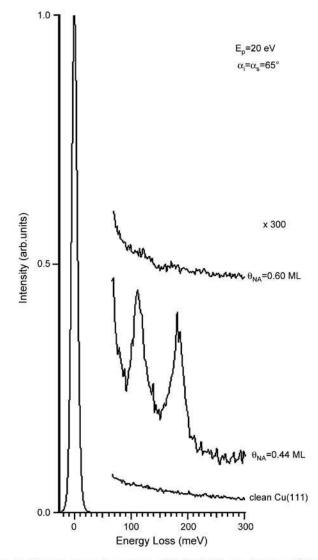
Fig. 1. Electron energy loss spectra of Na/Cu(111) as a function of the Na coverage.
