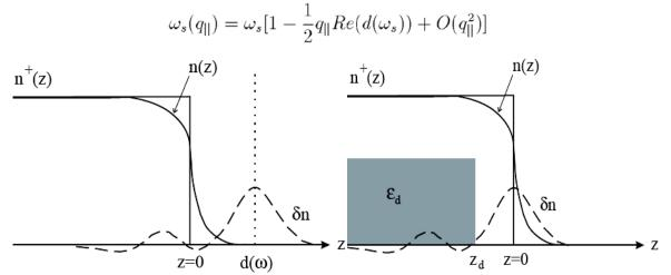
Figure 6: Position of the centroid of the dynamical screening charge  $d(\omega_s)$  with respect to the geometric surface.  $n^+(z)$  represent the positive jellium background, n(z) the negative charge density and  $\delta n$  the induced density. In the left panel the centroid of the induced charge lies outside the geometrical surface (z>0). But in the presence of a polarizable medium, represented by  $\varepsilon_d$ , the centroid is shifted inside the bulk (right panel).
