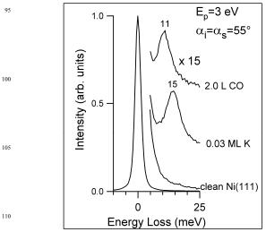
Figure 6: HREEL spectra for 0.03 ML K/Ni(111) deposited at 400 K. The K adlayer was successively exposed to CO at room temperature.
