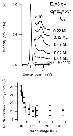
**Fig. 1.** (a) HREEL spectra of Na layers deposited on Ni(1 1 1) at 400 K (loss spectra were acquired at the same temperature). Loss peaks are due to the Na–Ni stretching vibration (b) behaviour of the Na-substrate vibration as a function of Na coverage.
