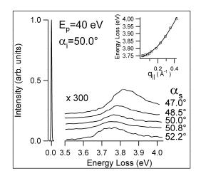
Figure 6: HREEL spectra for as-deposited 10 ML Ag/Ni(111) as a function of the scattering angle. In the inset the dispersion relation of the Ag SP energy is shown. A purely quadratic dispersion was found.
