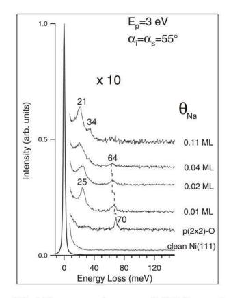
FIG. 4. Electron energy loss spectra of p(2-2)-O prepared at 400 K and after deposition of different amounts of Na at the same temperature.
