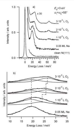
Figure 5. a) HREEL spectra of Ni(111) and 0.05 ML Na/Ni(111) exposed to  $O_2$  molecules at 400 K. b) Each curve is obtained using the same procedure as Figure 1 b.
