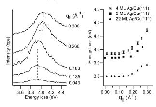
**Fig. 1.** (left) HREEL spectra for 5 ML Ag/Cu(111) (right) Dispersion of the SP energy for different Ag coverages. The lack of a dispersion before a critical wave-vector indicates that the SP is confined within Ag grains.
