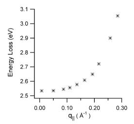
Fig. 3 Dispersion of the Au SP energy as a function of the parallel momentum transfer
