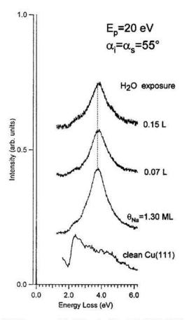
FIG. 4. HREEL spectra of Cu(111) and of  $\theta_{Na}$ =1.30 ML/Cu(111) exposed to water vapor.
