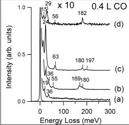
Figure 11: HREEL spectra at 300 K (at a fixed CO exposure of 0.4 L) for: (a) (3/2x3/2)-Na/Cu(111); (b) (3/2x3/2)-Na/Ni(111); (c) p(2x2)-K/Cu(111); (d) p(2x2)-K/Ni(111).
