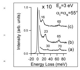
Figure 1: HREEL spectra for: (a) p(2x2)-O/Ni(111); (b) 0.04 ML Na coadsorbed with 0.10 ML of atomic O; (c) 0.04 ML K coadsorbed with 0.10 ML of atomic O. All spectra were normalized to the intensity of the 45 elastic peak and multiplied by the same factor.
