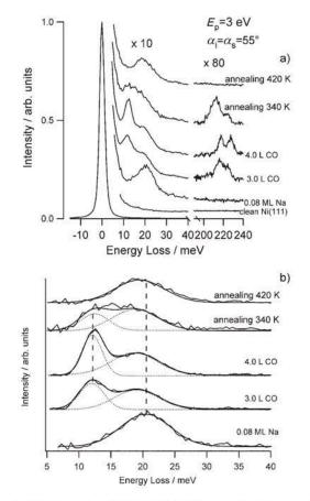
Figure 1. a) HREEL spectra of 0.08 ML Na/Ni(111) exposed to CO molecules at room temperature and successively annealed. Na was deposited at 400 K. b) Each curve is obtained by subtracting an exponential background and by fitting the resulting spectrum with Lorentzian lineshapes.
