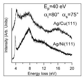
Figure 9: HREEL spectra of 10 layers of Ag on Ni(111) and Cu(111). The incident beam energy  $E_p$  was held constant at 40 eV and all spectra were recorded at an incident angle of  $\theta_i$ =80° with respect to the sample normal and with a diffusion angle of  $\theta_s$ =75°.
