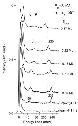
Fig. 5. HREEL spectra of  $c(4 \times 2)$ -CO prepared at 200 K and after deposition of different amounts of Na at the same temperature.
