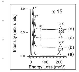
Figure 4: HREEL spectra for (a) 0.03 ML K adsorbed onto a Ni(111) <sup>30</sup> modified by the exposure of 1.0 L of CO. Successively, the surface was exposed to oxygen: (b) 0.2 L; (c) 0.5 L; (d) 2.0 L.
