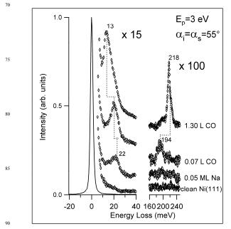
Figure 5: HREEL spectra for 0.05 ML Na/Ni(111) at 400 K for different CO exposures at room temperature.
