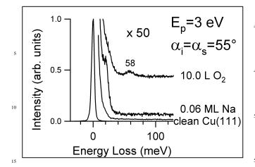
*Figure 3.* HREEL spectra of Na-doped Cu(111) surface and of Na+O/Cu(111). The loss feature at 22 meV is ascribed to Na-Cu vibration [23]. In Na+O/Cu(111) the presence of subsurface O is argued from the <sup>20</sup> appearance of the 58 meV peak. No on-surface species were revealed for Na-doped oxygenated copper.
