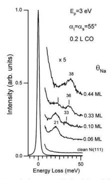
Fig. 4. HREEL spectra of various coverages of Na deposited onto the Ni(111) surface at 400 K and exposed to 0.2 L of CO at room temperature.
