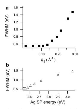
**Fig. 5** a (*top panel*) FWHM of the Au SP peak as a function of the parallel momentum transfer; b (*bottom panel*) FWHM of the Au SP peak as a function of the energy of the Au SP
