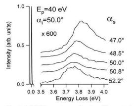
Figure 1 HREEL spectra as a function of the scattering angle for 10 ML Ag/Ni(111) at T = 300 K.
