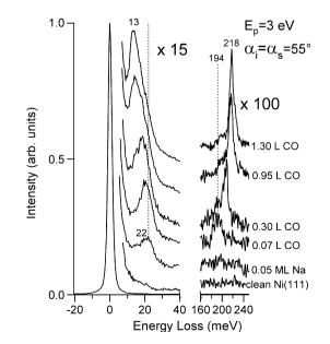
**Fig. 3.** HREEL spectra for 0.05 ML Na/Ni(1 1 1) deposited at 400 K for different CO exposures made at room temperature. Both the Na–Ni and C–O vibrational modes are shown.
