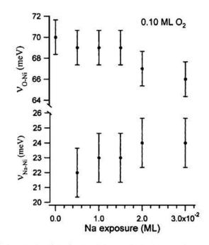
FIG. 3. Behavior of the O-Ni and the Na-Ni vibration energies as a function of Na exposure for an initial O-precoverage of 0.10 ML.
