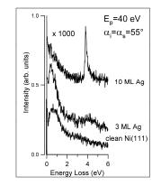
Figure 2: HREEL spectra of Ag/Ni(111) as a function of Ag coverage.
