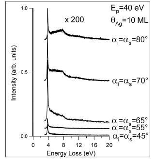
Figure 10: HREEL spectra of 10 ML Ag/Ni(111) as a function of the scattering geometry. Each spectrum was acquired in specular geometry.
