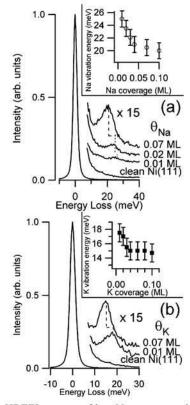
Figure 3. (a) HREEL spectra of low Na coverages deposited on Ni-(111) at 400 K (loss spectra were acquired at the same temperature). Loss peaks are due to the Na-Ni stretching vibration. The inset shows the behavior of the Na-Ni vibration as a function of Na coverage. (b) The same for panel a but for K.
