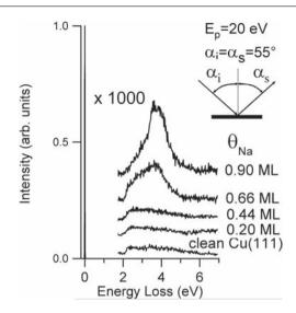
Fig. 1. HREEL spectra of Na/Cu(111) as a function of the alkali coverage. The incident beam energy  $E_p$  was 20 eV.
