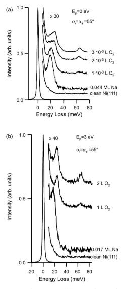
**Fig. 6.** (a) HREEL spectra for 0.044 ML Na/Ni(1 1 1) as a function of  $O_2$  exposures. Upon O adsorption, the Na–Ni vibration energy shifted from 21 to 26 meV. (b) Similar HREEL spectra for a lower Na precoverage, i.e. 0.017 ML.
