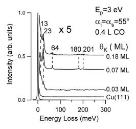
FIG. 2. HREEL spectra for various coverages of K deposited at 400 K on Cu(111) and exposed to CO at 300 K. Measurements were carried out at 300 K. A partial CO dissociation was argued by the presence of O-related modes.
