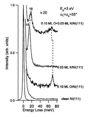
FIG. 6. HREEL spectra of (a) 0.03 ML of K deposited at 400 K onto the Ni(111) surface, (b) 0.10 ML O/Ni(111) at the same temperature, (c) 0.03 ML K coadsorbed at 400 K with 0.10 ML of O on the Ni(111) surface.
