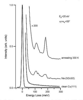
Fig. 2. Electron energy loss spectra for clean Cu(111) and for  $(3/2 \times 3/2)$ -Na/Cu(111) at 300 K and after a flash annealing at 330 K.
