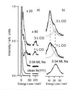
Figure 2. a) HREEL spectra of Ni(111) and 0.04 ML Na/Ni(111) exposed to CO molecules at room temperature. b) Each curve is obtained using the same procedure as Figure 1 b.
