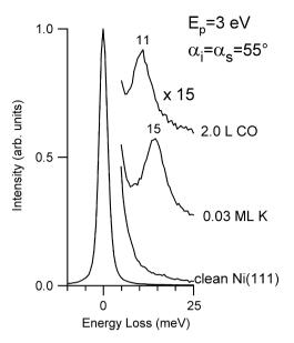
Fig. 4. HREEL spectra for 0.03 ML K/Ni(111) deposited at 400 K. The K adlayer was successively exposed to CO at room temperature.
