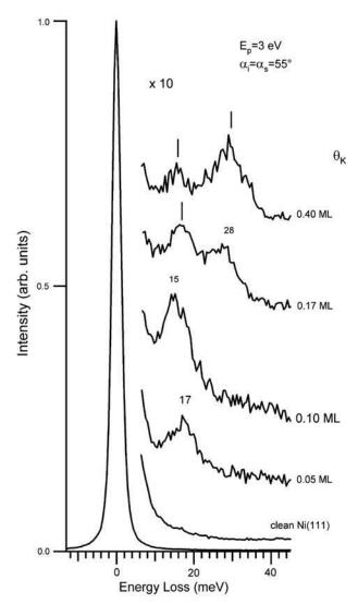
Fig. 5. HREEL spectra of various coverages of K deposited onto the Ni(111) surface at 400 K and exposed to 0.2 L of CO at room temperature.
