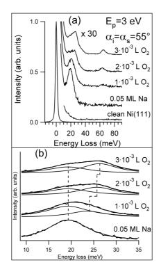
Figure 7: HREEL spectra of Ni(111) and 0.16 ML Na/Ni(111) exposed to  $O_2$  molecules at 400 K. (b) Each curve was obtained following the same procedure of Fig. 1b.
