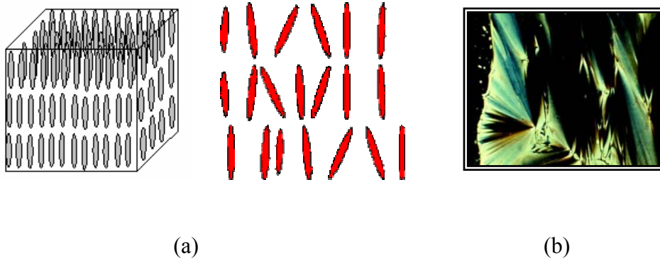
Fig.1.5. (a) Diagram showing the orientation of molecules in the Smectic A phase. (b) Typical texture of the Smectic A phase - the so-called “fans” consisting of “focal-conic” domains originated from the layered structure.
