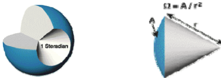
Figure 2.30: 4\pi steradian sphere on the right, cone with a solid angle of 1 steradian on the left
