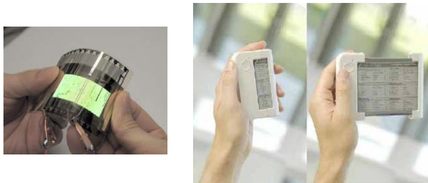
Figure 2.5: on the left, OLED on flexible substrate, source: Kyung Hee University; on the right, flexible display prototype.
