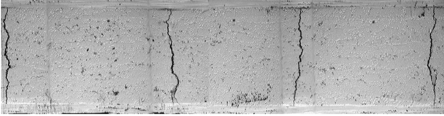
Fig. 1.3 Example of multiple matrix cracks observed in continuous fiber-reinforced laminates. Reprinted from [69].
