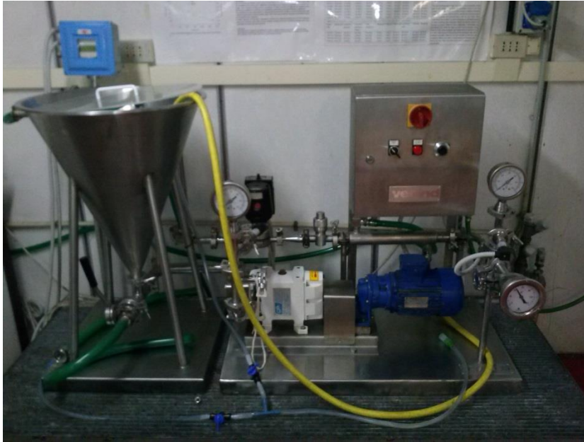
Fig. 3.20. Experimental set-up used for the clarification of raw press liquor by UF.
