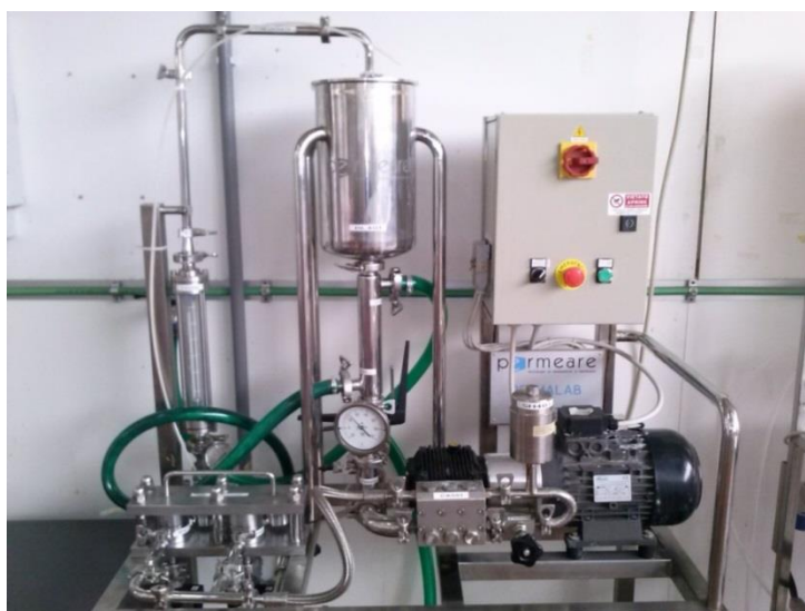
Fig. 4.1. Experimental set-up used for the NF with flat-sheet membranes.
