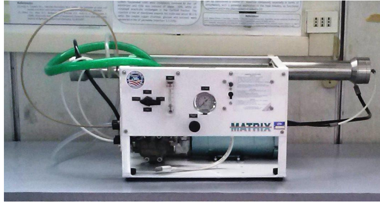
Fig. 4.6. Experimental set-up used for the NF of clarified orange press liquor with a spiral-wound membrane module.
