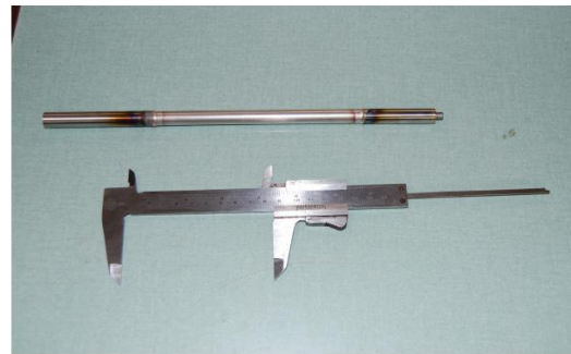
Figure 3. Dense tubular Pd-Ag membrane. This figure is available in colour online at www.apjChemEng.com .
