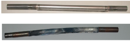
Fig. 8 – Dense Pd–Ag membrane used in POE reaction without catalyst: before and after reaction test.
