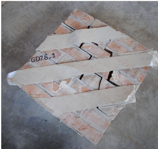
Figura 4.19 Quadri fessurativi: (a) GD7.8_1 (1); (b) GD7.8_1 (2)
