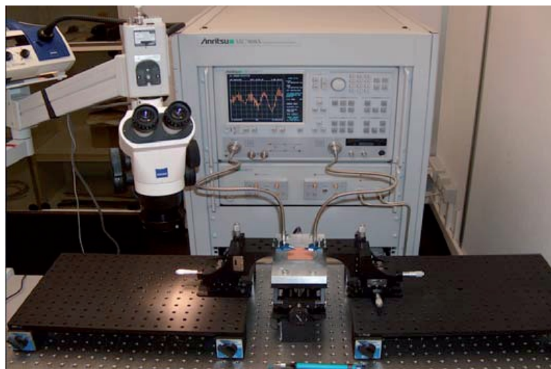
Fig. 2.25. Photograph of the test setup for the experimental validation of CBCPW on BCB substrate.
