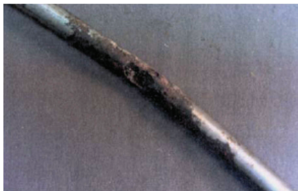
Fig. 3.7 – Pitting effect on a wire
