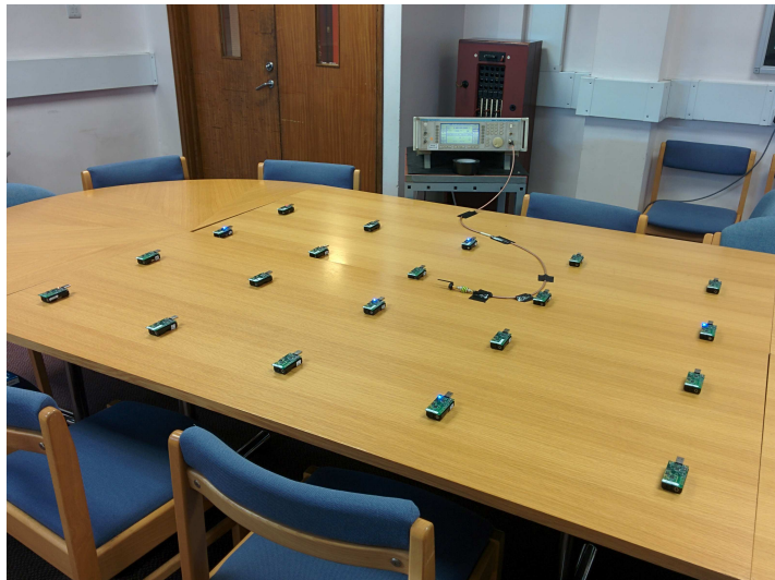
Fig. 5.11. Example of one of the rooms comprising our experimental setup. The 4 nodes at the right-most part of the image are used for monitoring purposes, while the RF signal generator, which acts to generate interference, is shown in the background.
