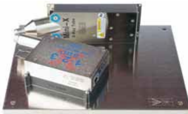
Figure 27: XRF portable setup
