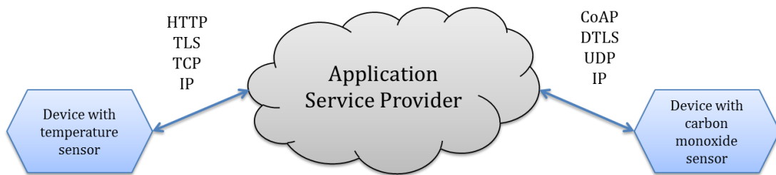
Figure 1.6 - Device-to-cloud communication model diagram.
