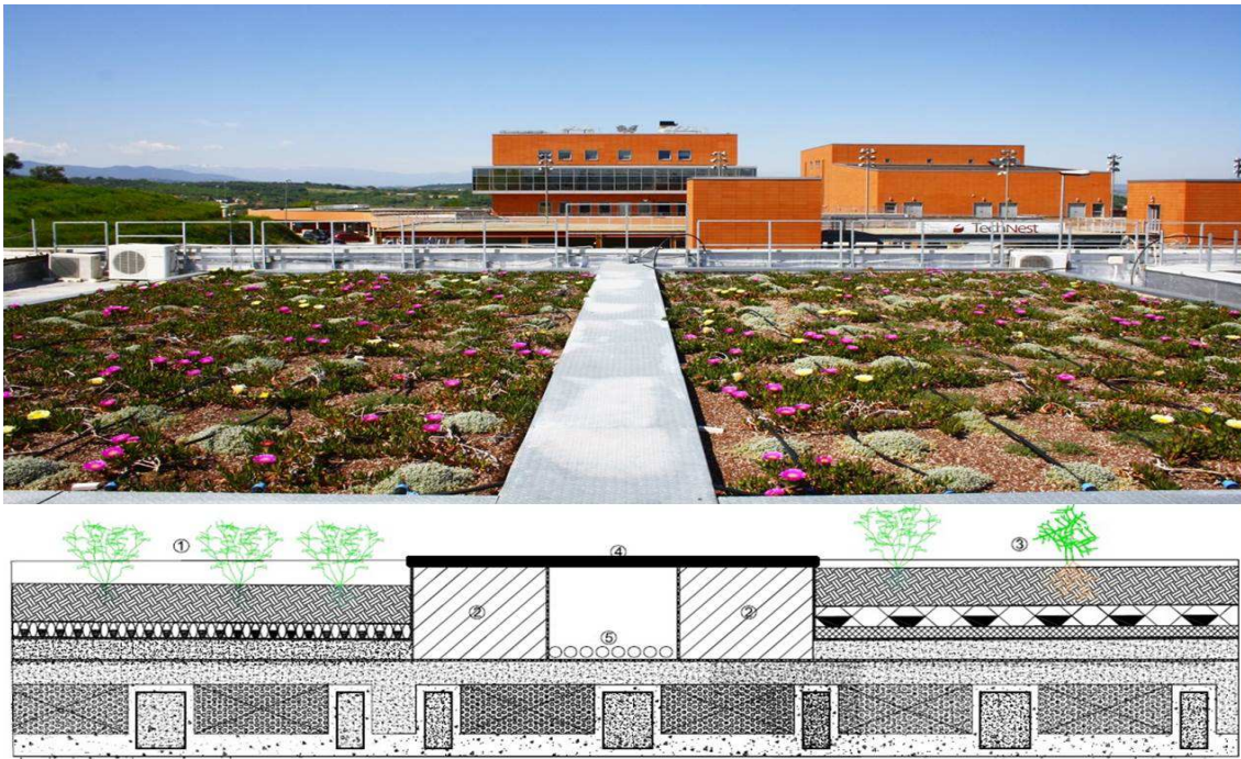
Fig. 5.3 A View and the Cross Sections of Sectors 1 and 2 of the Unical Experimental site; on the right and on the left respectively.
