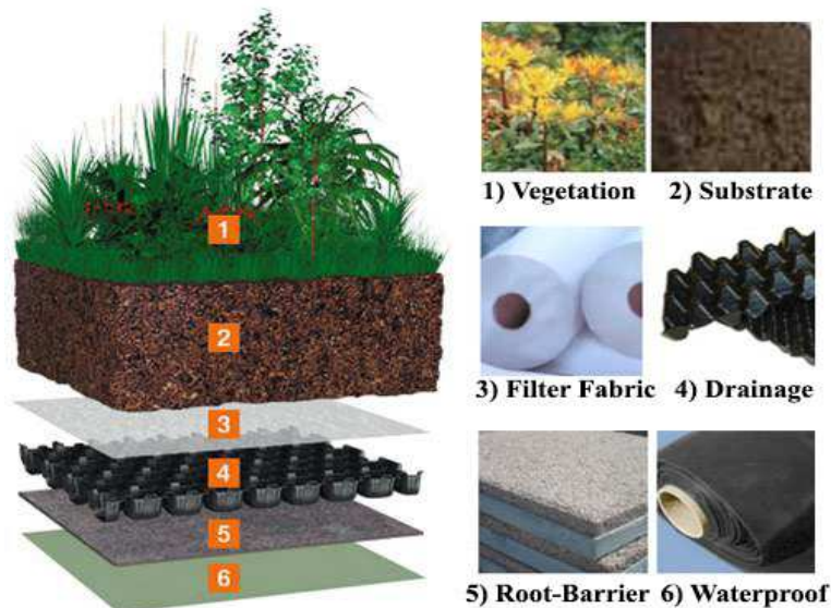
Figure 2.3 – Typical components of an extensive green roof
