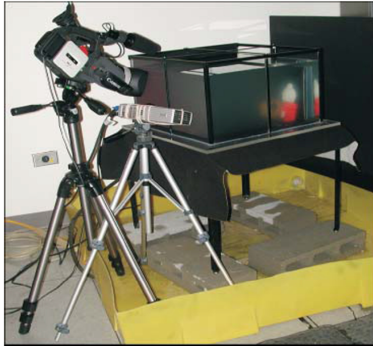
Fig. 1.11: Setup per la light stripe scanning
