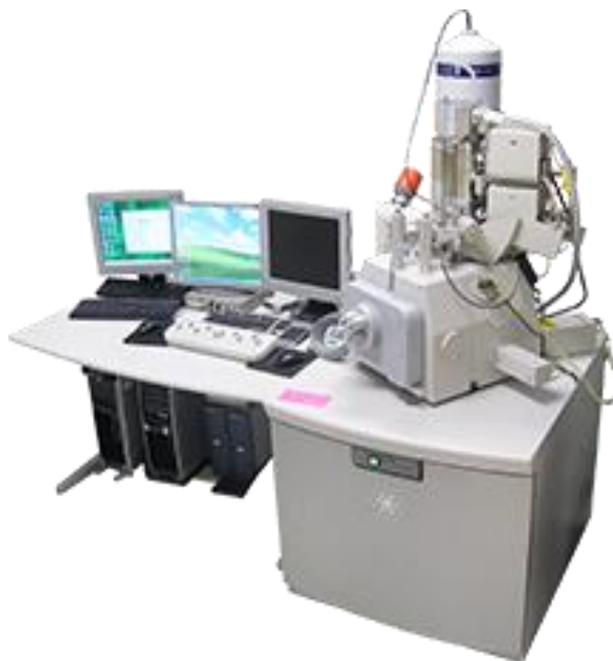
Fig. 26 Scanning Electron Microscope- FEI Quanta 200 Instrument
