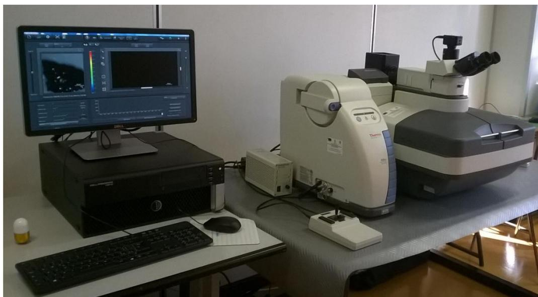
Fig. 29 Thermo Fisher DXR Raman microscope
