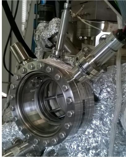
Fig. 8 LEED used for the experiments on this thesis
