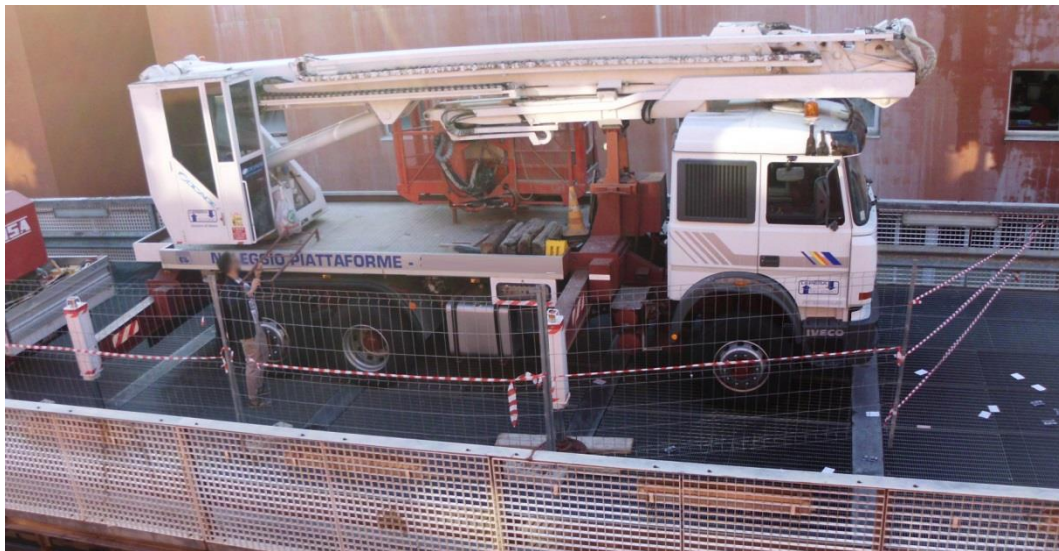
Figure 8.5: The truck elevator on the upper deck of the bridge.
