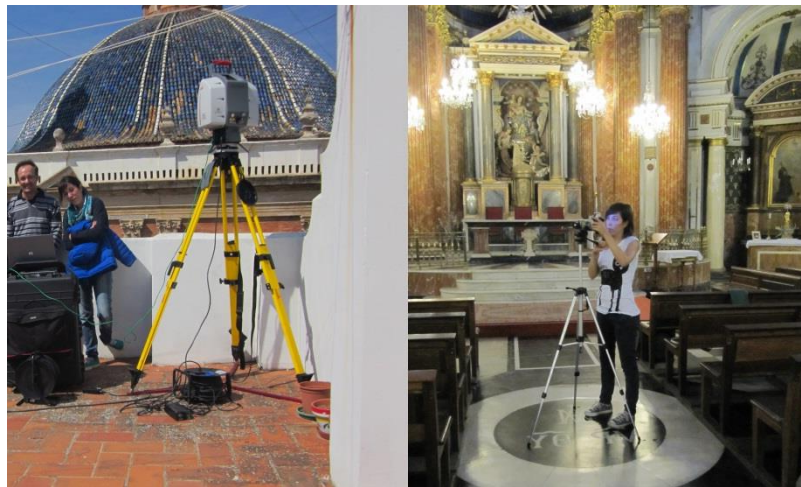
Figure 3.3: The survey with laser scanner and thermal camera.
