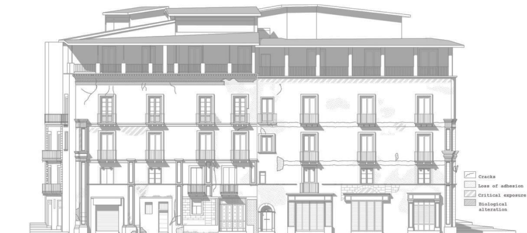
Figure 2.2: The degree of degradation and the crack pattern of the main façade.
