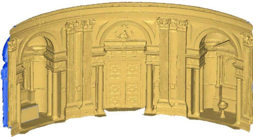
Figure 3.12: Level of detail of the mesh.
