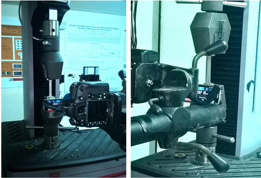
Figure 6.4: The apparatus for the shooting of the test on the aluminium specimen.
