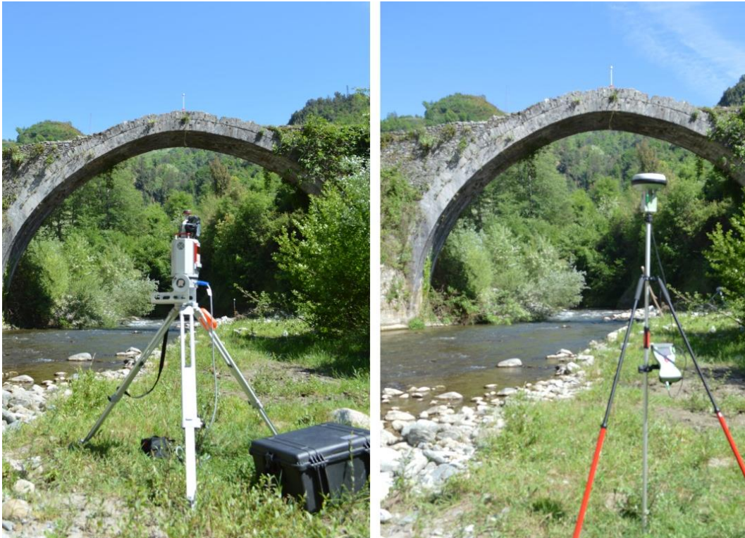
Figure 5.15 Survey of the Hannibal Bridge with Laser Scanners and GNSS receiver.
