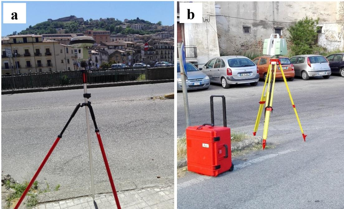
Figura 5-2. Ricevitore GNSS Leica GS15 (a) e Laser scanner terrestre Leica ScanStation P20 (b)
