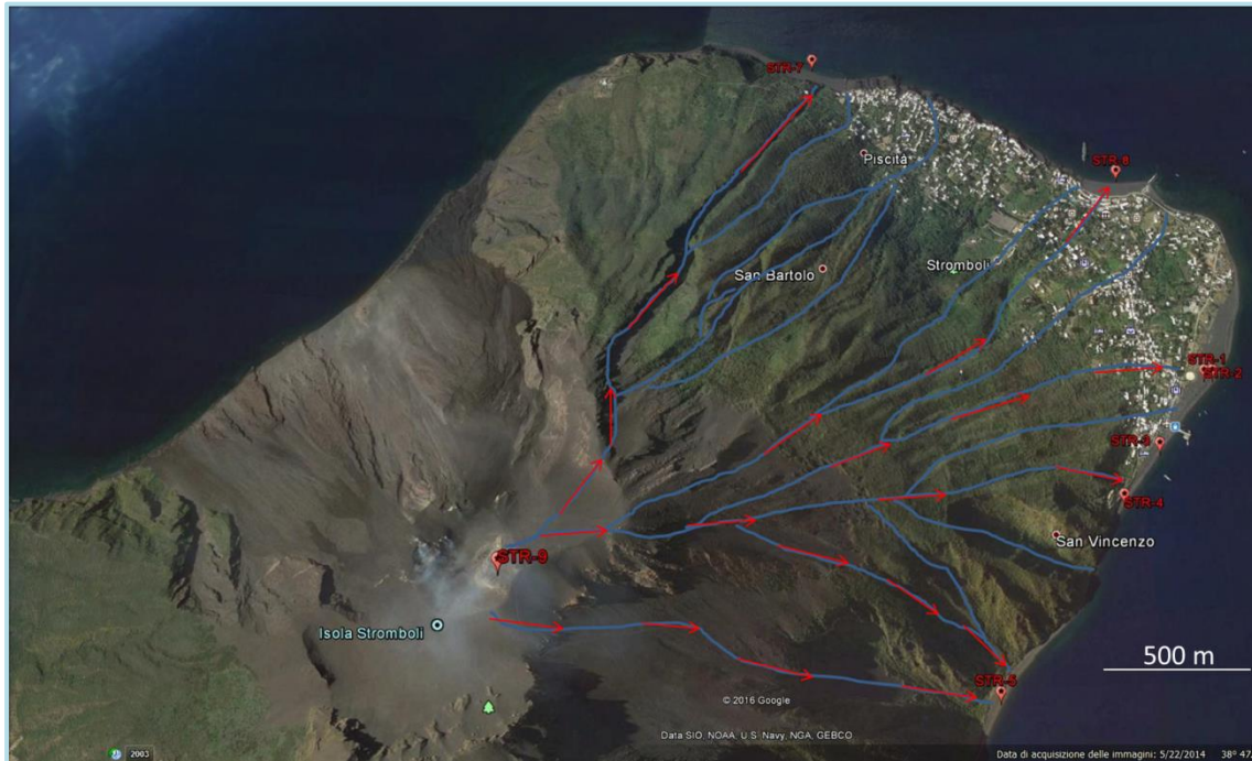
Figure 4.19 – Main Stromboli streams from craters to beaches (torrential transport). High relief, it goes from 924 to 0 m.a.s.l. in short distances (about < 1.7 km minimum and < 3,5 km maximum).
