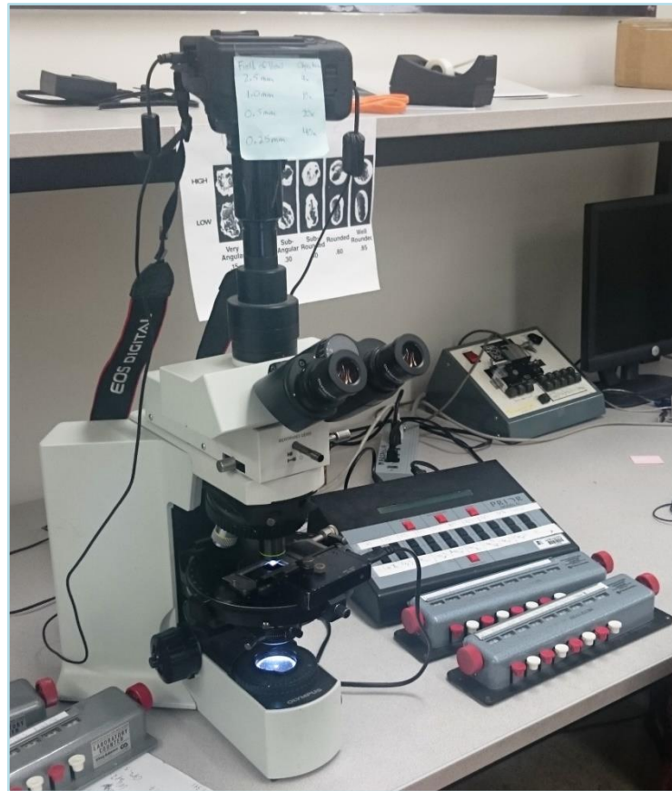
Figure 4.13 – Polarizing microscope connected to a point counter with automated stepper-stage.
