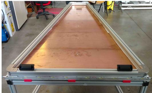
**Figure 3.24:** Frame used to press mesh-frames and mesh-corners on the drift panel during the glue curing.
