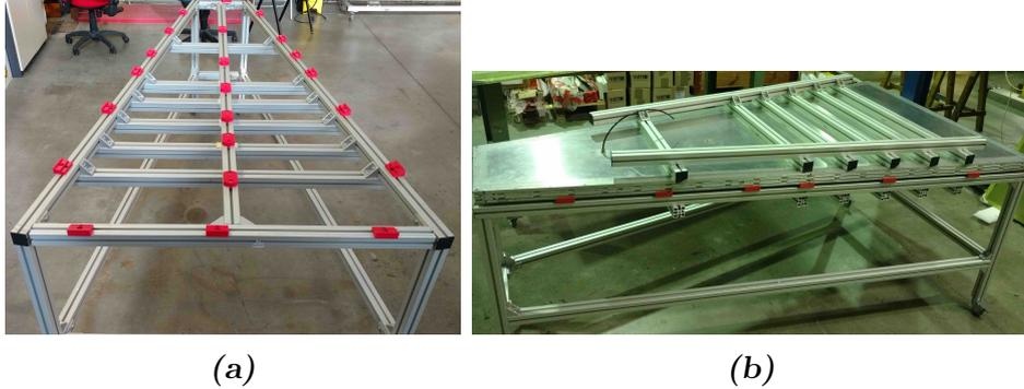
**Figure 3.19:** Finalization-table for the gas tightness test with all its elements: aluminum structure with the reinforce bars at the interconnection position (3.19a), vessel and exoskeleton (3.19b).
