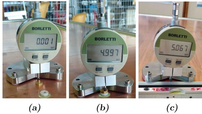
**Figure 3.26:** The micrometer on its holder during three different measurement: Fig. 3.26a shows the zeroing on the brass disk; Fig. 3.26b shows the height measurement of a interconnection drift spacer; Fig. 3.26c shows the measurement of the mesh-frame height.
