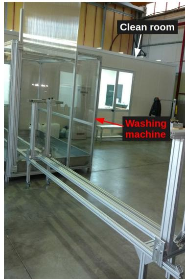
**Figure 3.31:** The washing cabin operation: the mesh is placed inside the cart and pushed inside the cabin. The cabin door is then closed and the washing start usign high pressure washer. Finally, the mesh is moved in the clean room through a door directly connected to the clean room. Designed by Alessandro Miccoli.
