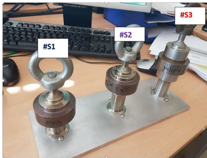
Figure 7.9. SMA-based prototype chambers used for irradiation test.
