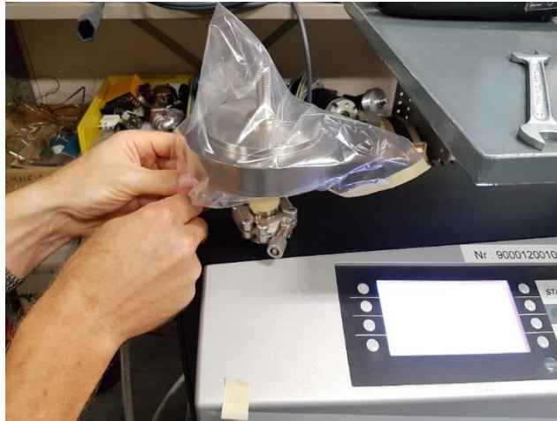
Fig. 5.23: operator performing a leak detection test
