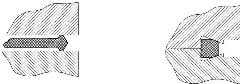
Figure 3.6: Seal detail of a diamond cross section aluminum seal between flat flanges (left) and of standard CF flanges using corner-crush gasket(right)
