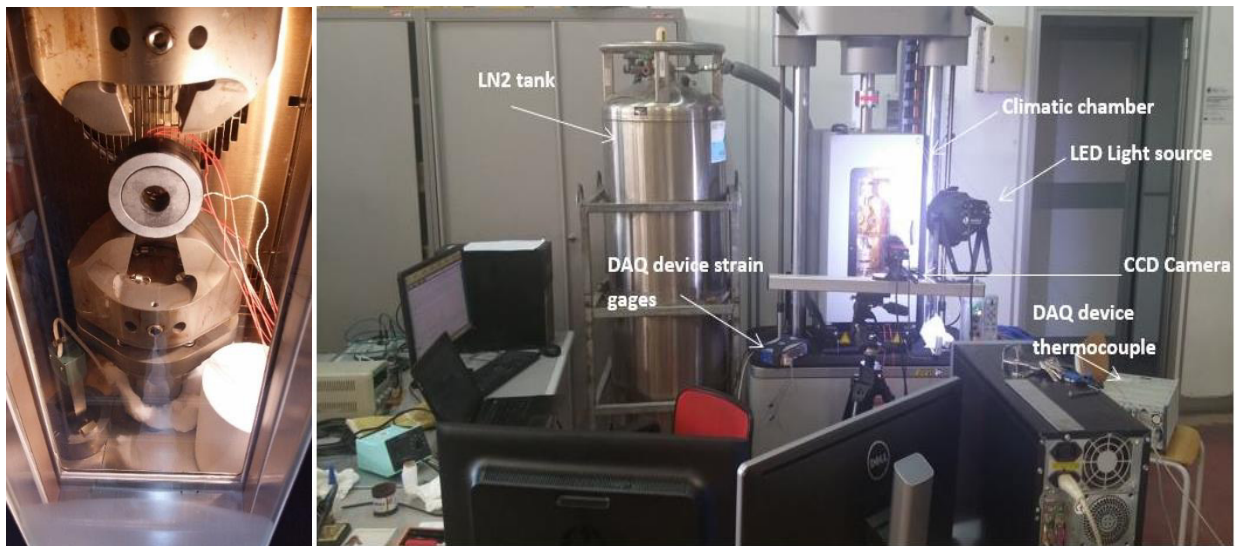
Figure 5.9: (a) Assembled SMA/steel rings for DIC and strain gauge measurements and (b) complete experimental setup for thermomechanical testing of SMA rings
