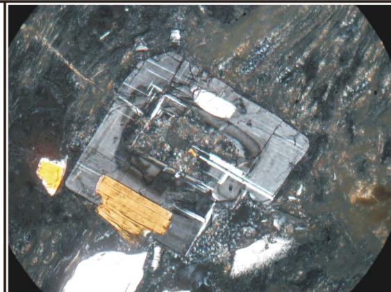
B) Neo-volcanic plagioclase (euhedral) including biotite grain. Note the strong zonation, to which correspond, at the center, alteration from zeolites minerals. Southern Rhodopes (10x)
