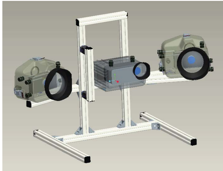
Figure II.7: Virtual prototype of the underwater 3D scanner.
