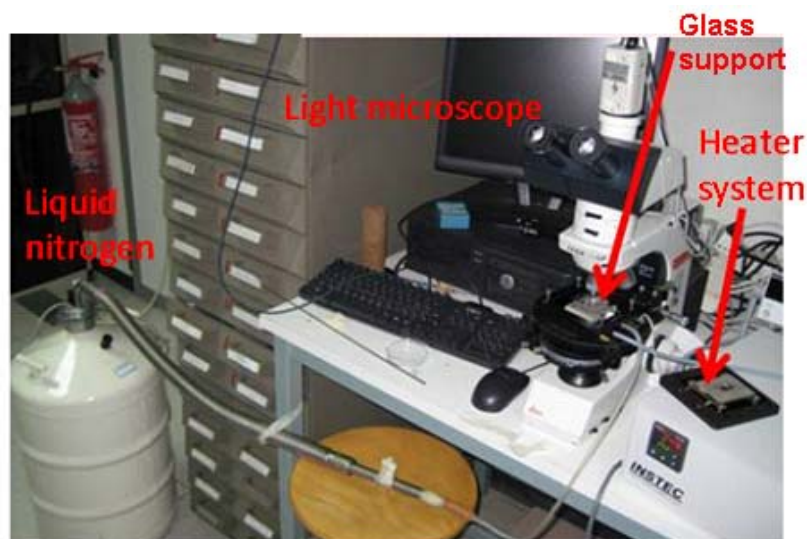
Figure 6.2 Experimental set-up for the study of shape phase transition in DMPC GUVs.
