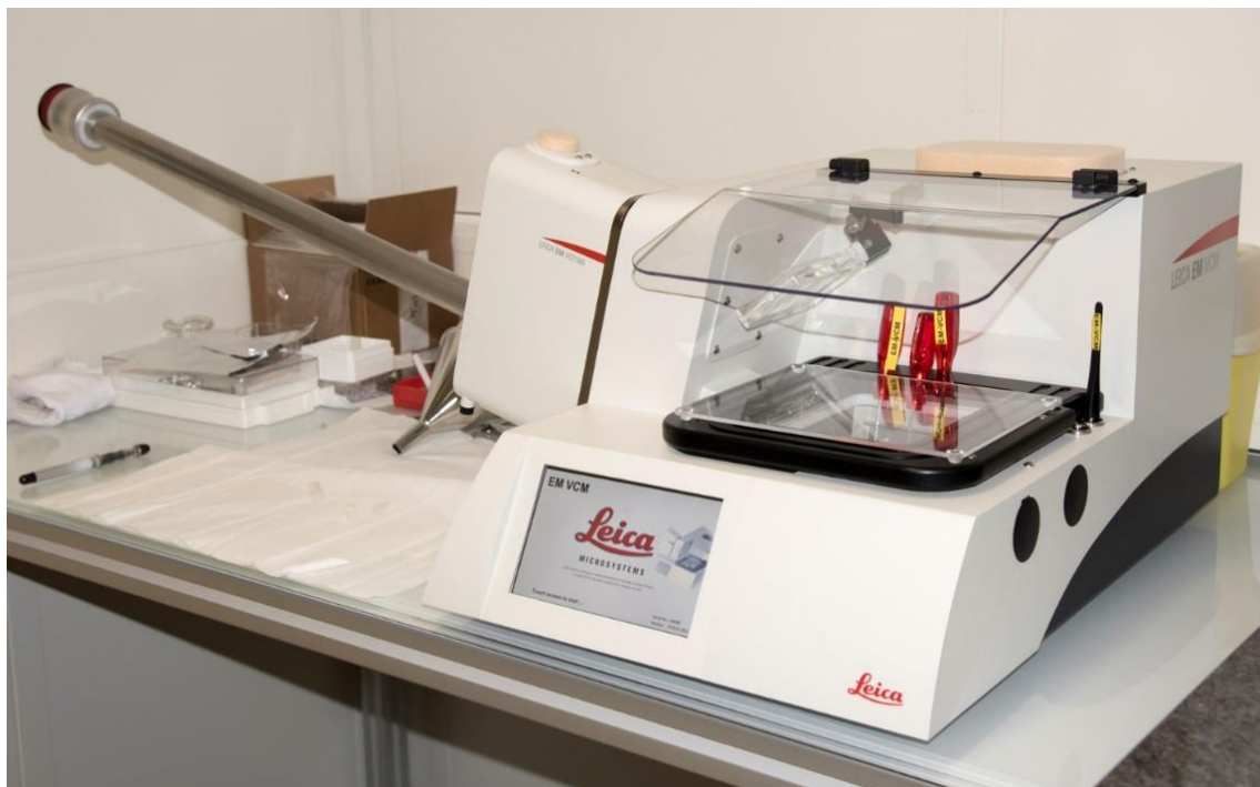
Figure 5.2: Cryo loading chamber and transfer system.
