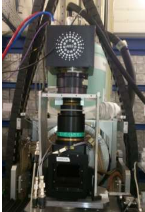
Figure 115: Detector couple with the 1:3.6 optic.
