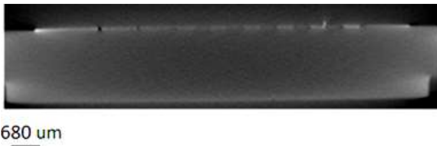
Figure 80: 2D \mu\text{CT} cut of MOSFET #1 after n-irradiation
