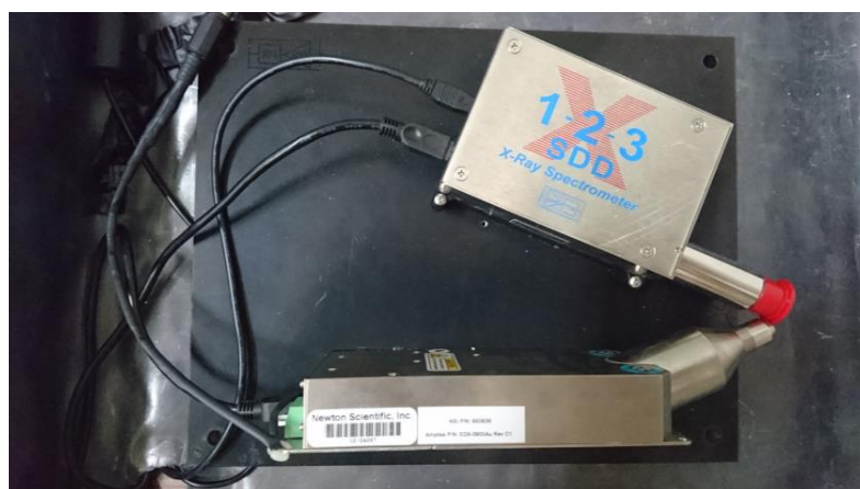
Figure 7 - XRF portable setup
