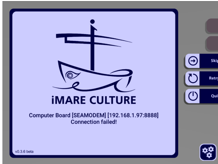
Figure 34. The user can decide to skip the connection to the computer board.
