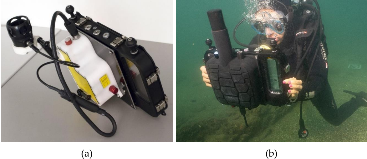
Figure 29. The two new acoustic localization systems coupled with the underwater tablet. (a) The USBL system; (b) the SBL system.
