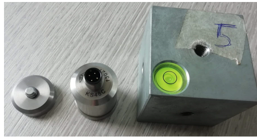
Figure 2.7: KS48C-model: magnetic attack, accelerometer, nut
