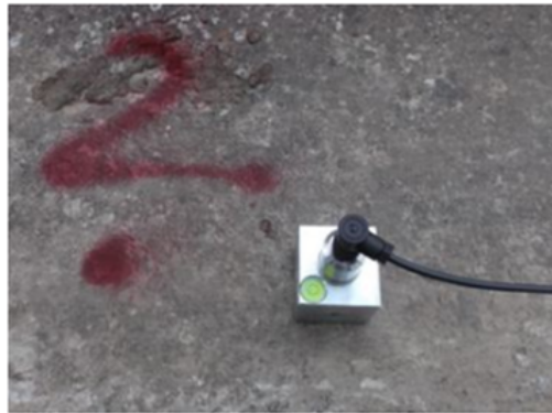
Figure 4.11: Acceleration trasducer uniaxial with base
