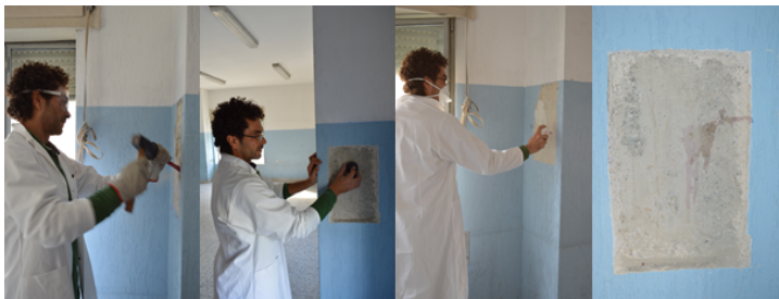
Figure 5.6: Test of concrete's carbonation: Plaster removal; Surface sanding; Test for phenolphthalein
