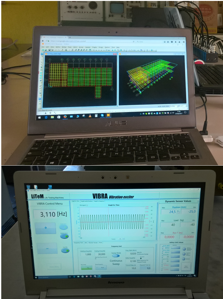
Figure 5.31: ITI A. Monaco: finite element modeling in SAP2000 and software screen for input data forcing
