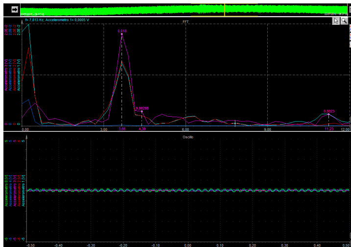
Figure 4.24: Fiume di Mare Bridge: experimental frequencies that activated the 2nd mode of vibrating
