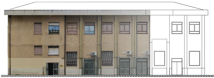
Figure 5.5: Reconstruction of an elevation from orthogonalized images
