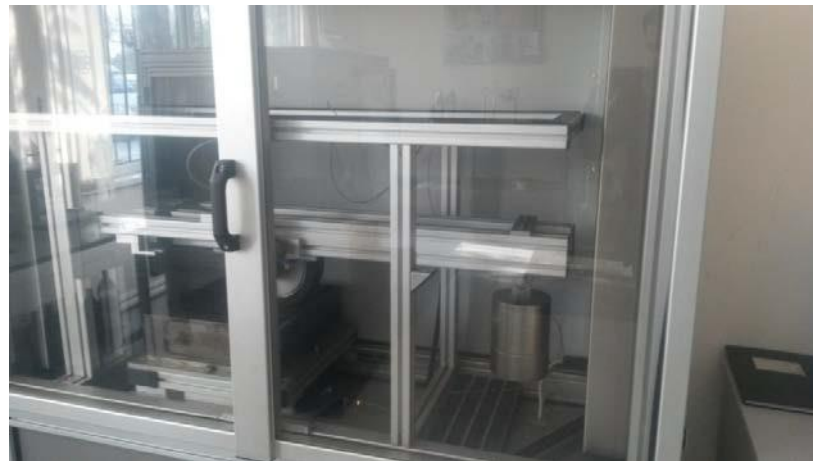
Figure 3.4 Installation of the Hamburg Wheel
