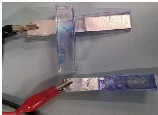
Figure 9. The intact cathode (connected to the black caliper) and the consumed anode.
