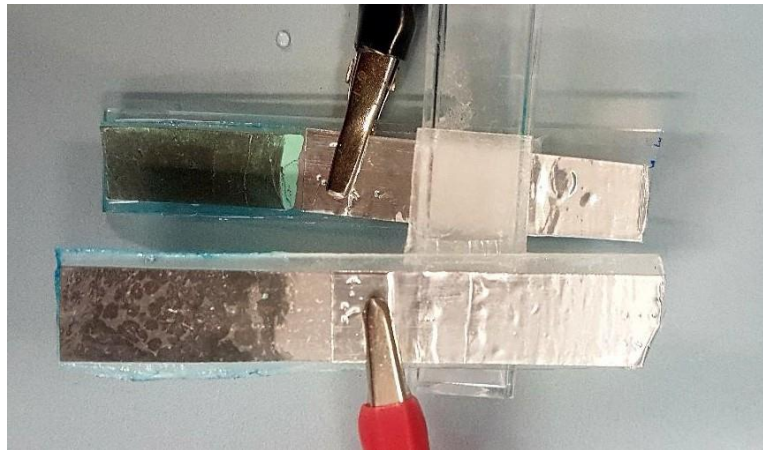
Figure 12. Anode (up) and cathode (down) after 330 of EC test.
