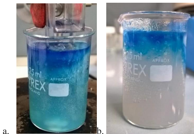
Figure 11. Solution after a. 30 minutes and b. 1 hour of EC treatment.
