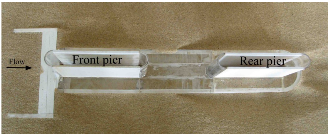
Fig. 201. Scour pattern at the end of test U8
