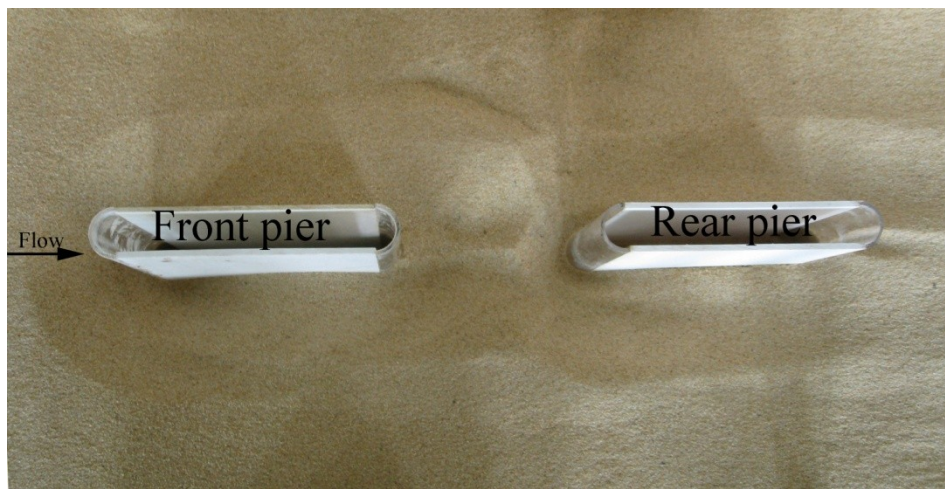
Fig. 195. Scour pattern at the end of test U6
