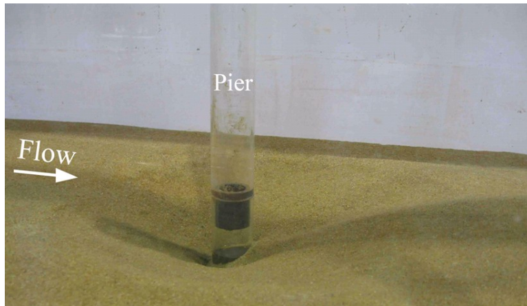
Fig. 71. Scour hole at the end of test S0
