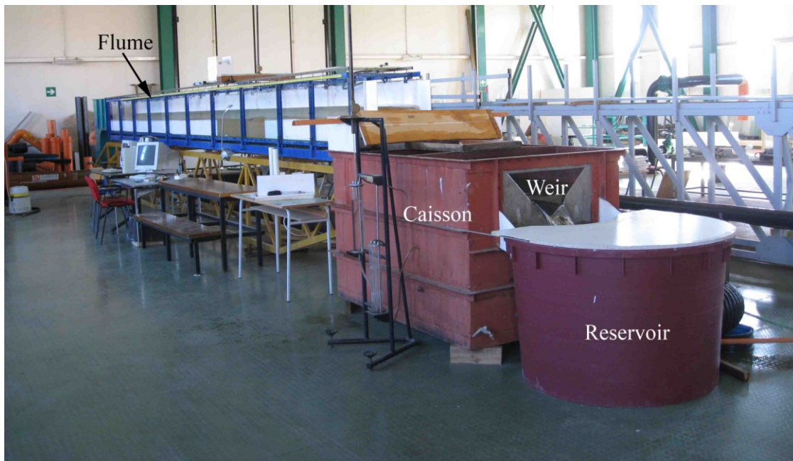
Fig. 44. General view of the flume
