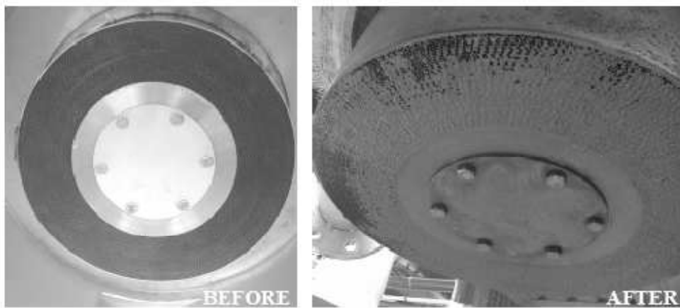
Figure 4.10: Rotating particle separator before and after testing at ECN
