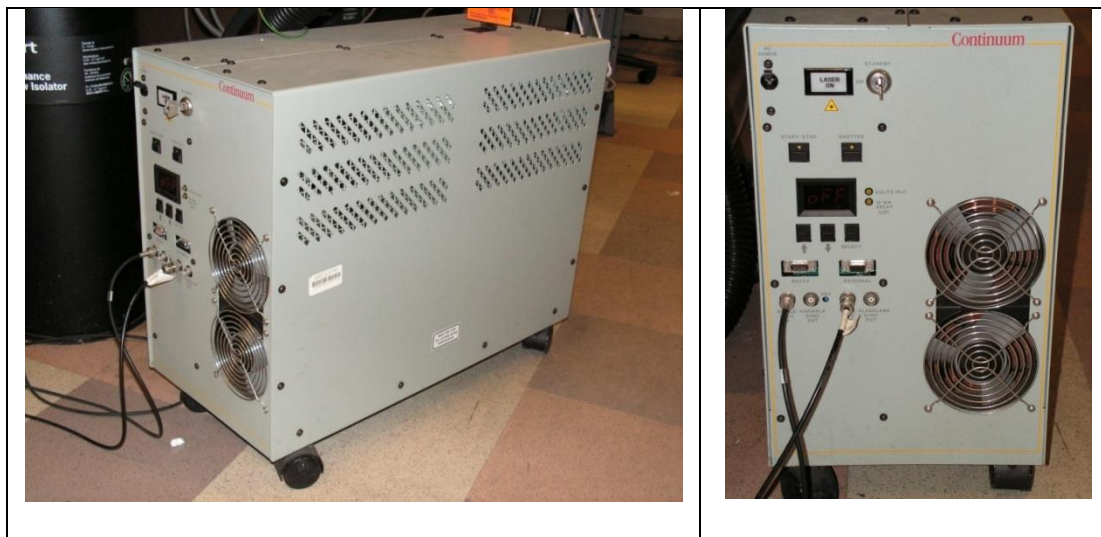
Figure 5.1: Continuum® Surelite SLI-20 Q-Switched laser (power supply unit).
