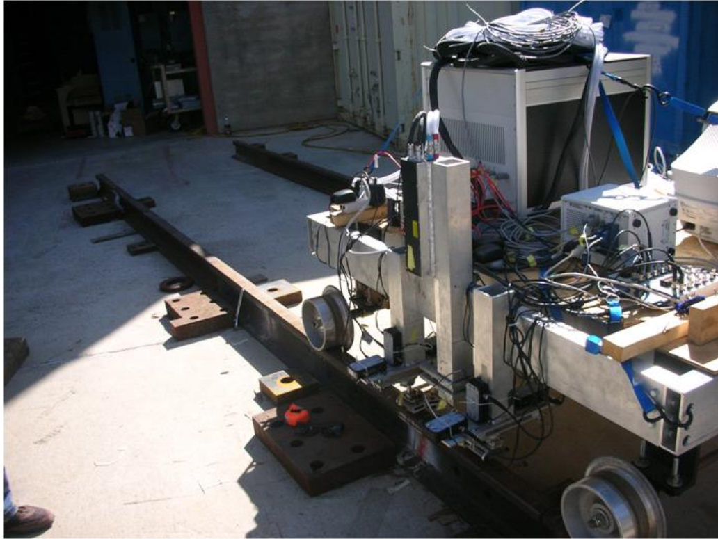
Figure 4.26: Rail defect detection prototype deployed on the rail track mock-up at UCSD
