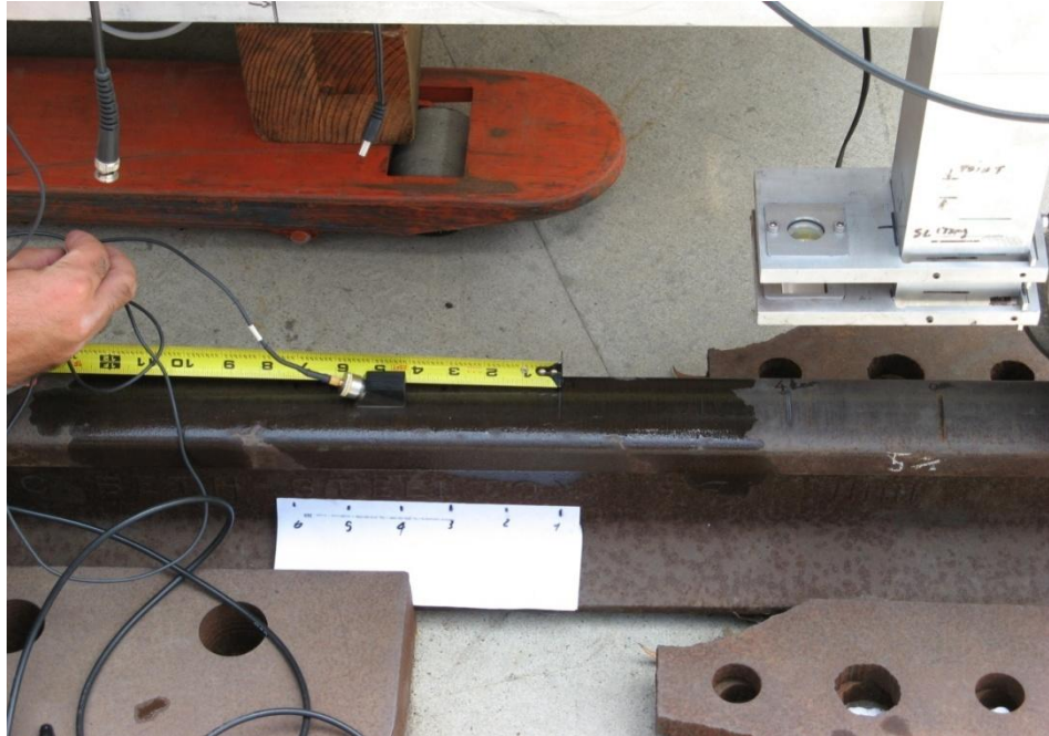
Figure 4.7: Test setup: laser excitation and transducer spacing in proximity of the 5% H.A. reduction surface defect
