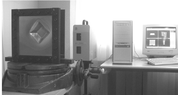
Figure 2.8: The laser based scanning system set-up
