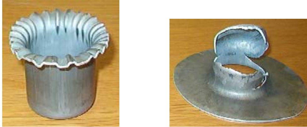
Figure 3.13: Wrinkled and broken components.
