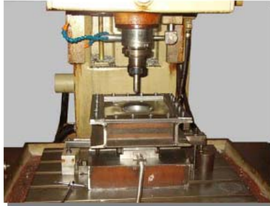
Figure 2.3 – The SPIF equipment for forces measurement on CNC machine
