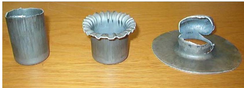
Figure 3.6: Experiments carried out with a LDR= 2.63: sound (a), with wrinkling (b) and broken parts (c).
