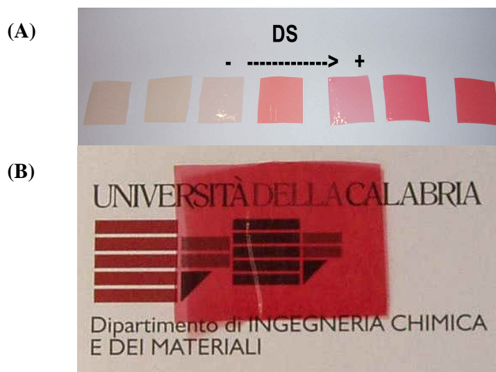
Figure 38. Photograph of SPEEK-WC membranes with various DS ((A) in order from left to right: 0.10, 0.22, 0.36, 0.60, 0.70, 0.80, 1.04) and a composite membrane containing H_3PW_{12}O_{40} ((B) DS=0.8)
