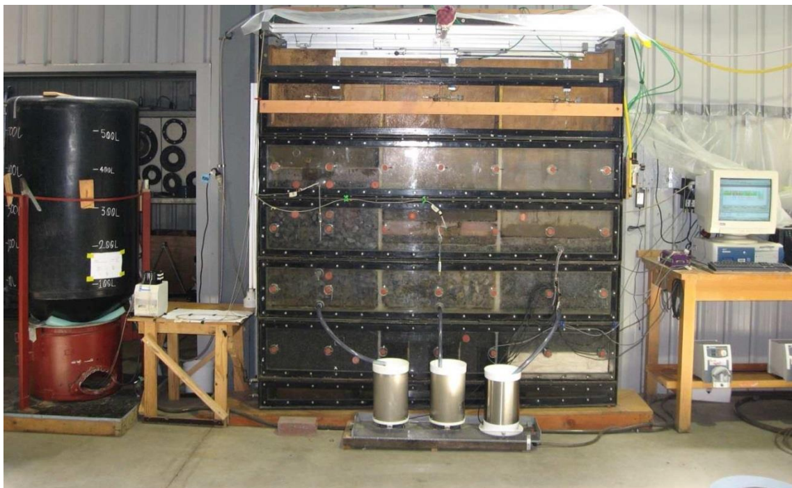
Fig. 5. 23 - The Monash University Melbourne experimental rig for the comparison of (from left to right) PA, HP and PP (Yong et al., 2011).
