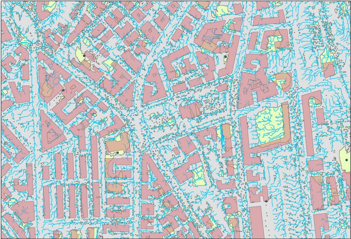
Fig. 2. 11 - Use of DEMs without superimposed buildings can lead to common errors like delineation of ponds and overland flow path within them.
